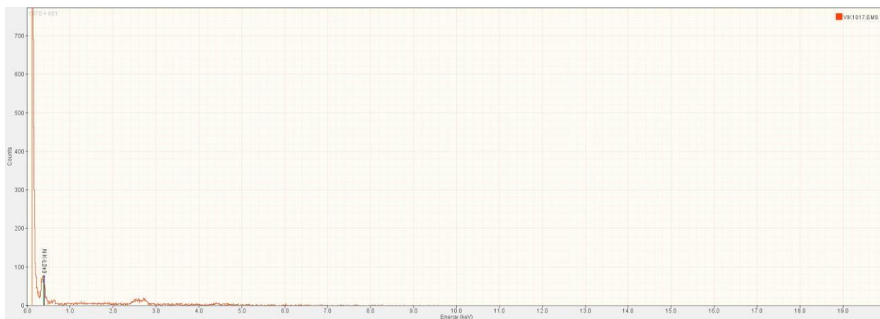
Figure 20- EDS spectrum of the drug loaded titanium nanotubes. The spectrum shows a N peak at 0.392 keV.
