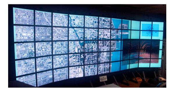
Figure 3. LambdaVision, EVL's first generation wall-sized display, 105 megapixels in resolution.
