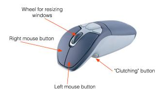
Figure 14. The Gyromouse (made by Gyration) is used for enabling interaction from a distance.
