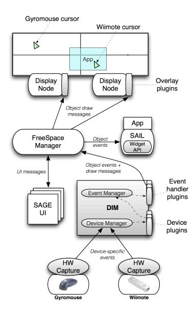
Figure 10. Direct Interaction Manager integrated with SAGE. Device Manager handles multiple physical interaction devices, Event Manager performs event distribution for device events, individual event handlers manage the logic and overlays manage the drawing of objects. The components in gray are all a part of the Direct Interaction Manager.
