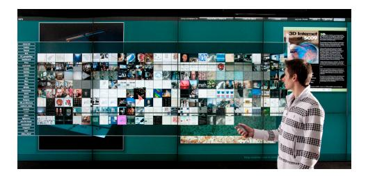
Figure 19. The media browser, developed using SAGE widgets, is a tool for easily browsing and showing multimedia files on large high-resolution displays.
