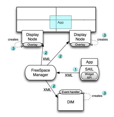
Figure 11. The three-step process of creating an application widget, a button in this case.
