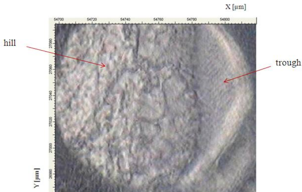
Figure 5.2 ATR-FTIR optical image and mark of the Ge crystal recorded on a striated pattern (hill and trough) on the articulating surface of the retrieved tibial insert.
