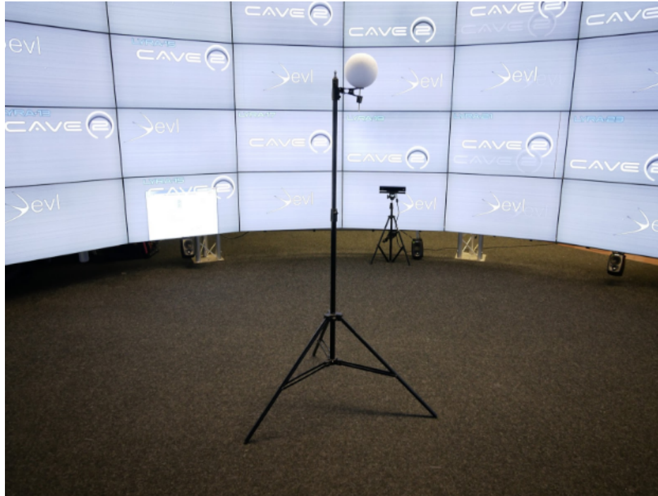
Figure 5: In front, tripod with 15 cm diameter Styrofoam sphere used to calibrate the environment. Behind, Kinect sensor reallocated to meet Microsoft's requirements.
