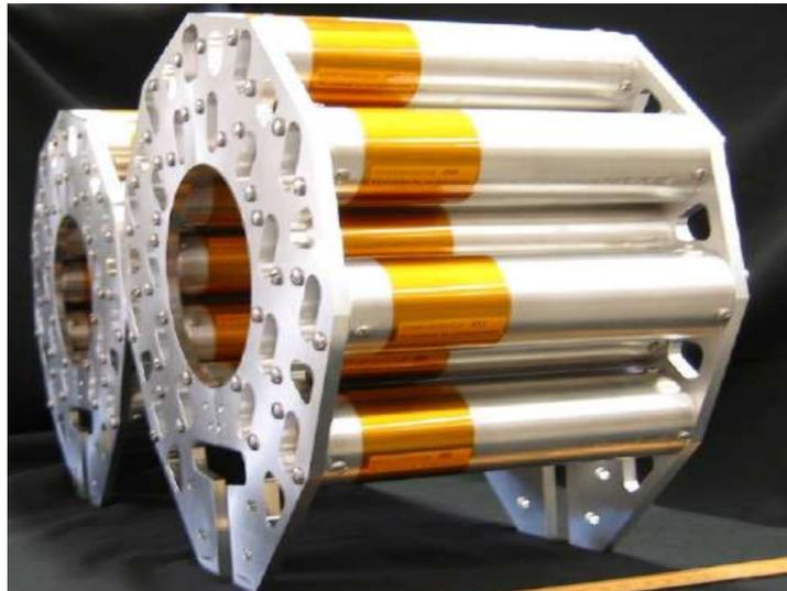
Figure 36: STAR Vertex Position Detector (VPD) [68].
