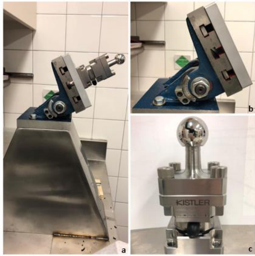
Figure 5: a) Elevated test set-up with taper, force sensor, and angle plate. b) Varying angle plate. c) 3-dimensional force sensor (Kistler 9347C) with taper and femoral head components
