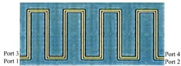
(b) CMOS 3dB directional coupler using meander edge-coupled synthetic transmission lines. (Source: reference [21] Fig. 1.)
