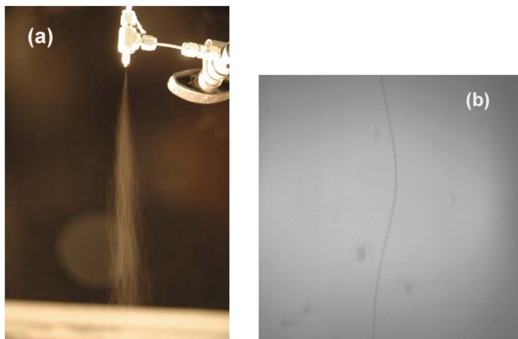
Fig. 10.2. Solution blown polymer jet at 25 bar. (a) The envelope and (b) a snapshot.
