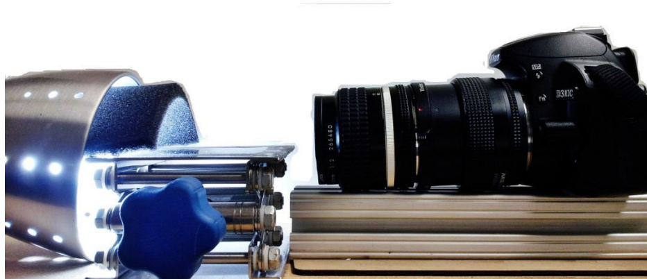
Figure 9. Image showing custom apparatus used to measure water contact angle
