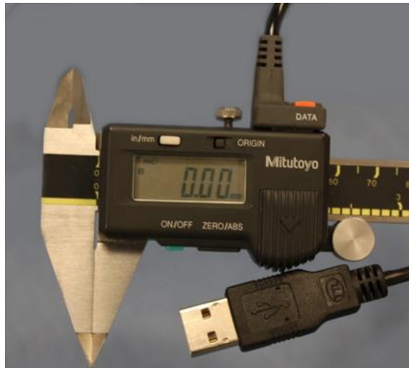
Figure 2. Mitutoyo Digimatic® caliper with USB data output switch
