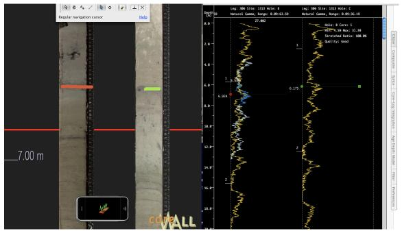
Figure 27. Using Corelyzer (left) with Correlator (right) to do visual stratigraphic correlation. A scientist could initiate the connection to Corelyzer from Correlator. Correlator would pass core data information to Corelyzer so high-resolution core images could be loaded inside Corelyzer. The scientist could then use visual features of core images to assist tie points correlations in the Correlator.
