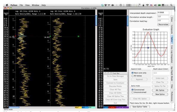
Figure 26. A Correlator session screenshot. Two gamma ray attenuation (GRA) data plots from two different holes were loaded in the left-hand-side. The user could pick feature corresponding points from each of the plot denoting that they were the same feature. The right-hand-side similarity graph could be used to evaluate how good the correspondence is as moving these two points' positions along the depth.
