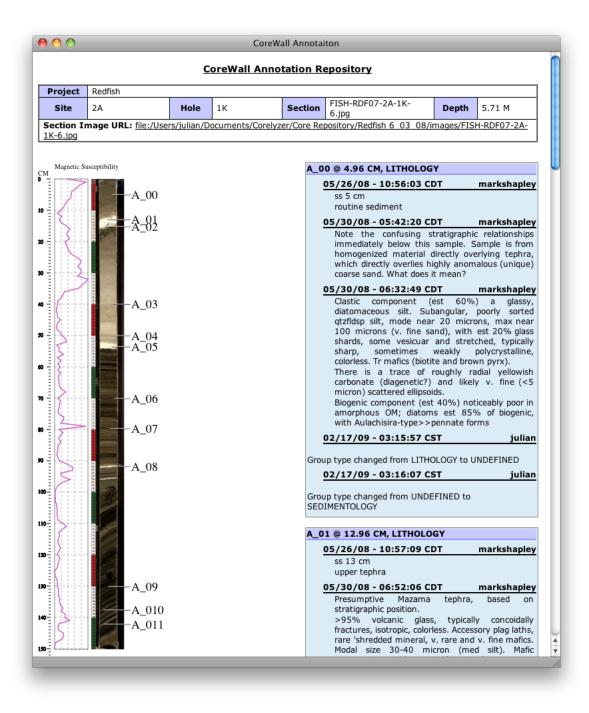
Figure 23. A barrel sheet output example. This is an example of a scientist using the CoreWall as a research note-taking tool. Top part of the sheet contains metadata about where the core section is from. On the left hand side, core section image and magnetic susceptibility plot are co-registered in depth with annotations highlighted. On the right hand side, it shows freeform notes threaded in time.
