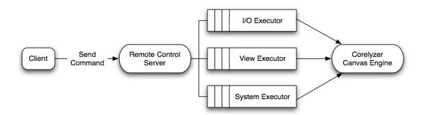
Figure 28. Corelyzer remote control server thread pool architecture
