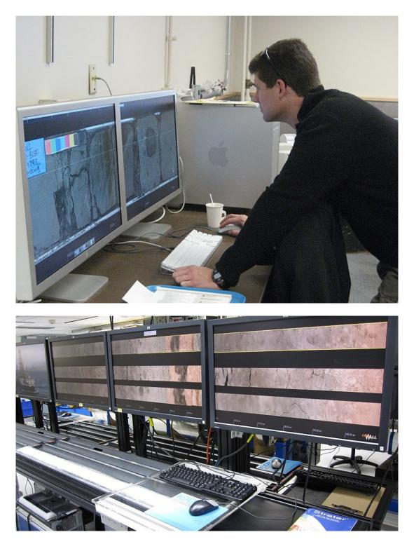
Figure 12. CoreWall setups in different hardware configurations. Above: Dr. Tomas P. Wagner using the CoreWall during ANDRILL 2006 season in the Crary Laboratory at the McMurdo station, Antarctica. Photo by Joshua Reed. Below: The multi-panel CoreWall system on IODP U.S. JOIDES Resolution scientific drilling vessel.
