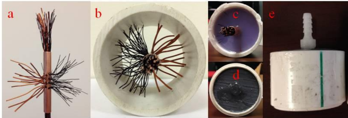
Figure 5-2: (a) Big and small wires used for interconnected porosity network in phantom regions. (b) Wire network placed in rigid plastic cylinder. (c) Ecoflex solidification around wire network in cylinder. (d) Back side of cylinder with rigid plastic disk glued in place. (e) Additional plastic disk with barb fitting is glued onto other end of cylinder once wires and perforated copper tube are extracted from the solidified Ecoflex.
