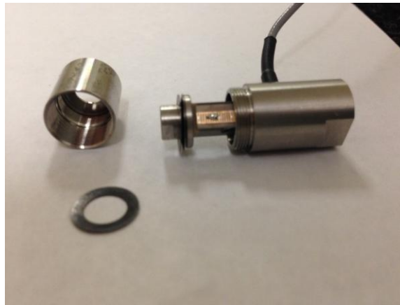
Figure 4-4: Piezoelectric stack used to vibrate phantoms in MRE experiments.
