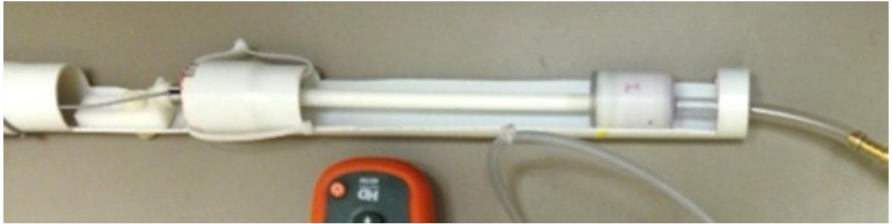
Figure 4-3: Multilayer phantom mounted in MRI insertion platform and connected to piezoelectric actuator. Plastic hose inserts into phantom for pore pressure control.
