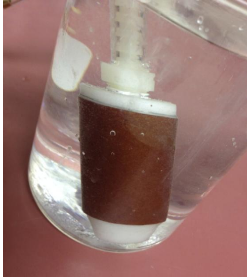
Figure 3-2: Completed multi-layer phantom is shown placed in water for visual air bubble leak pressure testing before experiments.
