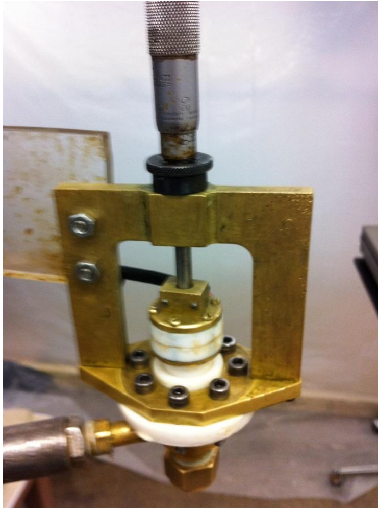
Figure 3.5 Needle type atomizer
