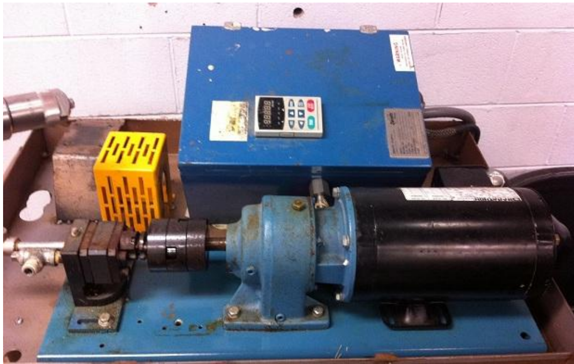
Figure 3.7 High pressure pump connections and frequency controller
