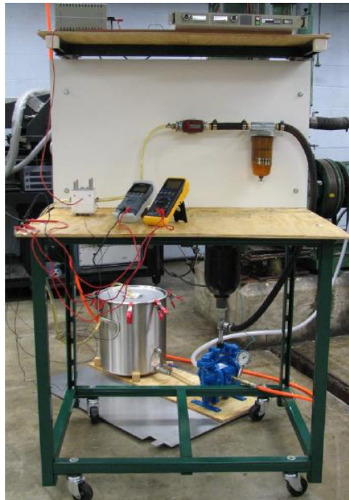
Figure 4.9 The complete flow rig with blade type charge injection system
