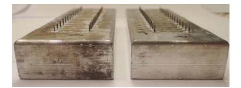
Figure 2. Aluminum blocks with 0.80 mm diameter pins set 19.05 mm apart.
