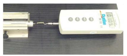
Figure 6. Chatillon (Largo, FL) DFM 10 Force Gauge and latex elastic being stretched to 19.05 mm.
