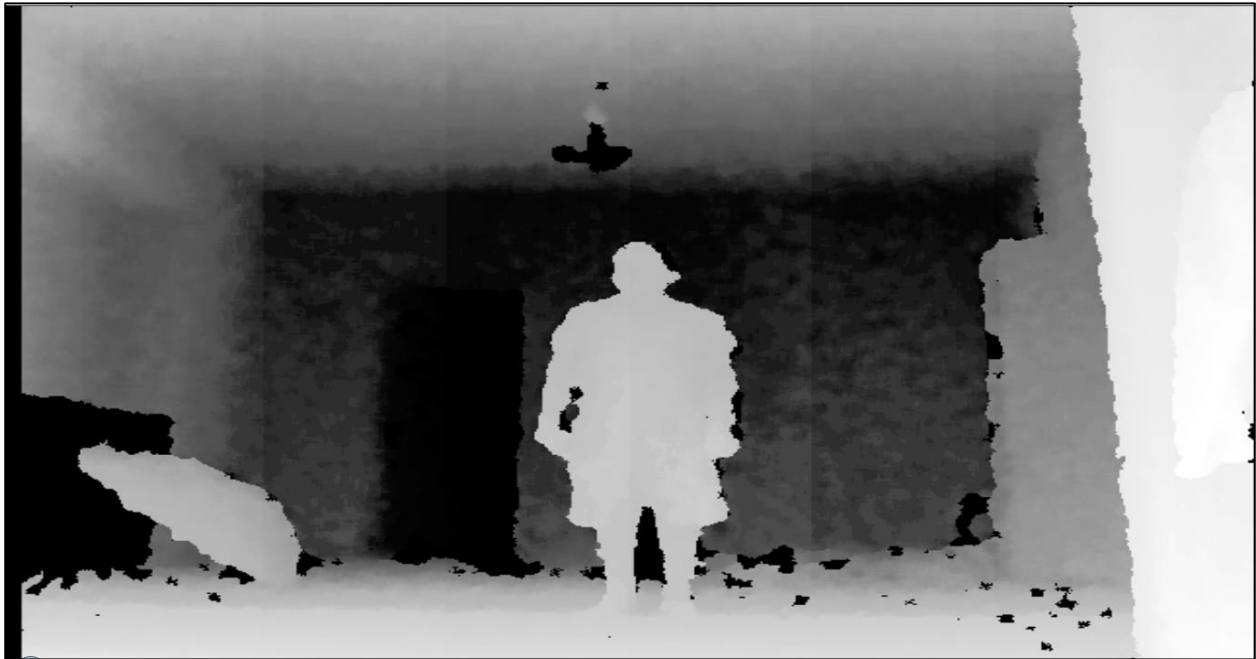
Fig 5. Output From The Depth Camera Of The Kinect.
