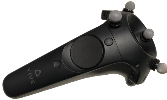
(a) Vive controller with retro-reflective markers
