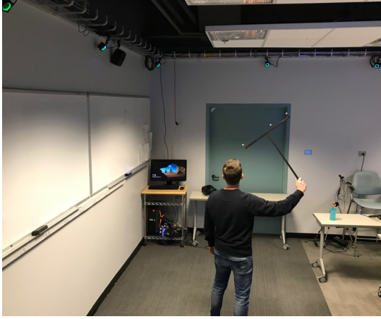
(a) Person performing the wanding calibration
