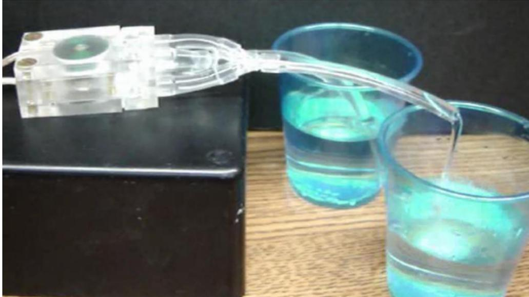
Figure 43 - Micropump v2.0 pumping distilled water.
