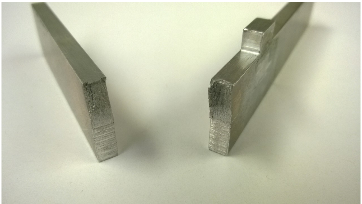
Figure 73. The failure section of the fatigue test II
