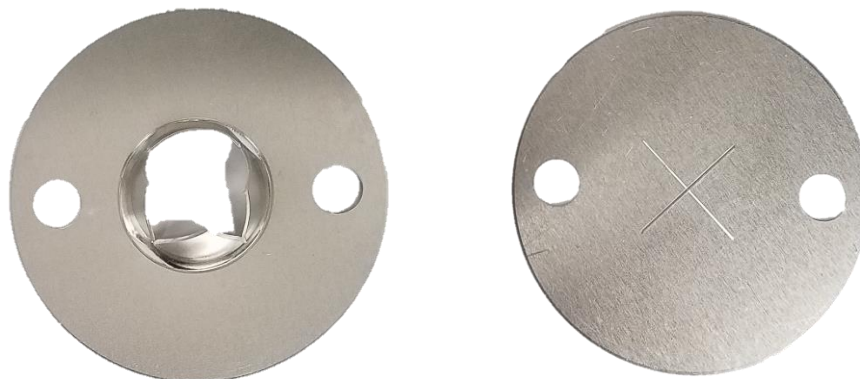
Figure 2: Example of typical 3003 grade aluminum diaphragms used for the experiments. A burst diaphragm is shown on the left, and an unused diaphragm on the right.
