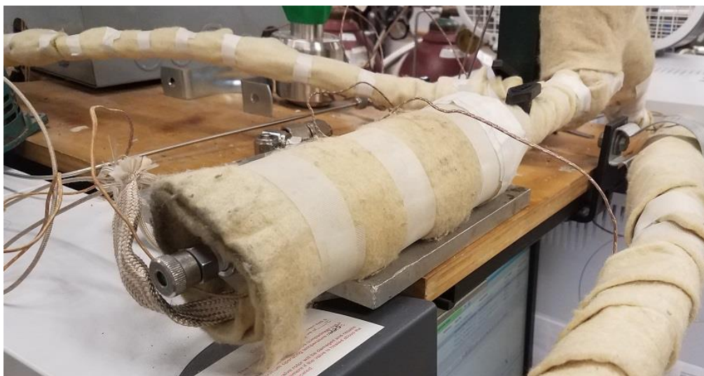
Figure 6: Recent picture of the heated 300 cc vessel used for GC calibration.
