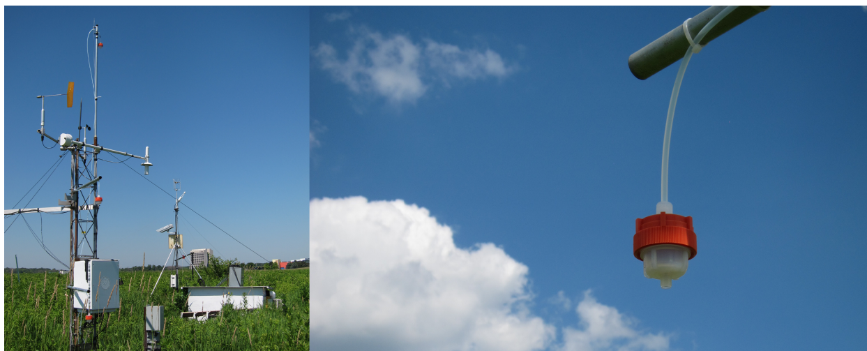
Figure 7. Sampling inlets at the Fermi tallgrass prairie. Eddy covariance tower (left) with four filtered inlets (three pictured, the fourth is obscured by the grasses) photographed on June 19, 2016. Detail of a hanging inlet (right).
