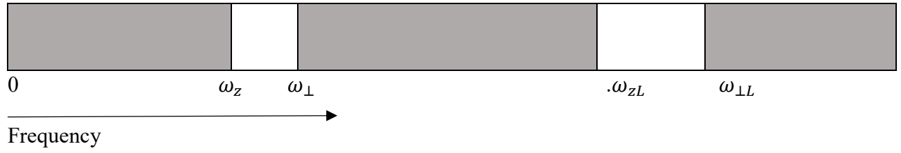
Figure 16 Shaded region showing the range of frequencies for which \varepsilon_{||}\varepsilon_{\perp} > 0 .
