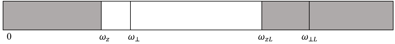
Figure 17 Shaded region showing the range of frequencies for which \varepsilon_{||} > 0 .
