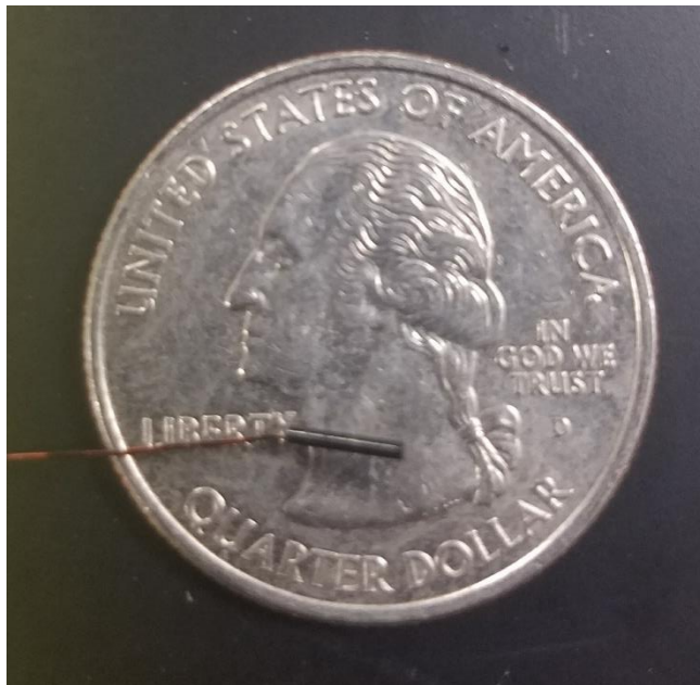
Figure 11. Example of the thermistors used in this study, with a U.S. quarter dollar coin for scale. Thermistor dimensions are provided in the text.
