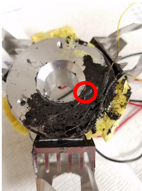
Figure 7. A view of the inferior side of the ECR. The black liquid is the thermally conductive epoxy. This ensured that heat was efficiently transmitted to the ECR thermistor (shown in the red circle). This portion was later insulated with neoprene.
