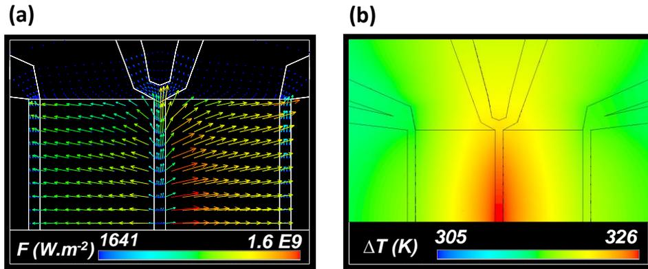
**Figure 5. Finite Element (FE) Simulations and Analyses.** (a) Vector plot of the thermal flux in a half-model FE simulation of the thermometry device, showing asymmetric heat dissipation through grain and GB regions. (b) Temperature distribution in the FE model.
