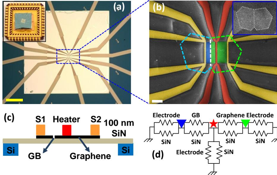
**Figure 4. Electrical Thermometry Platform for Investigation of Individual Graphene GBs.**
