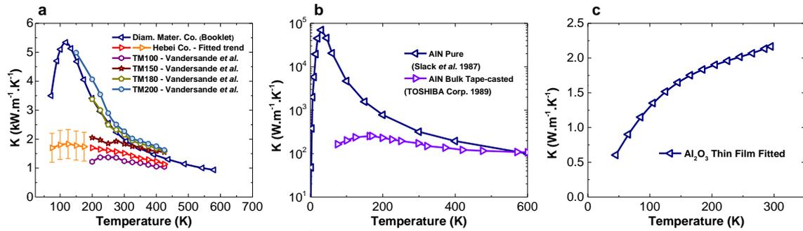
**Figure 26. Thermal Conductivities of The Materials vs. Temperature.** (a) Diamond[238], (b) AlN[243], (c)  $\text{Al}_2\text{O}_3$  thin film.
