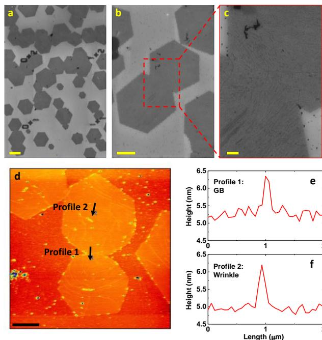
**Figure 1. Topographic Characterization of Graphene GBs.** (a-c) SEM images of the uniform and well-stitched graphene GBs. It is clear that overlapping or disconnection does not exist in the merging region of the flakes. Scale bars in (a), (b), and (c) are 20 μm, 10 μm, and 2 μm, respectively. (d) The AFM topography image of two merged graphene GBs. The scale bar is 5 μm. (e-f) the height profiles across the GB and across a wrinkle in the single crystalline grain.
