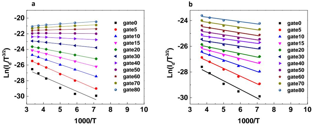
**Figure 31.** Arrhenius Measurements at  $V_{sd} = 1$ V for Different Applied  $V_g$  for (a) MoS<sub>2</sub>-graphene (b) MoS<sub>2</sub>-metal transistors.
