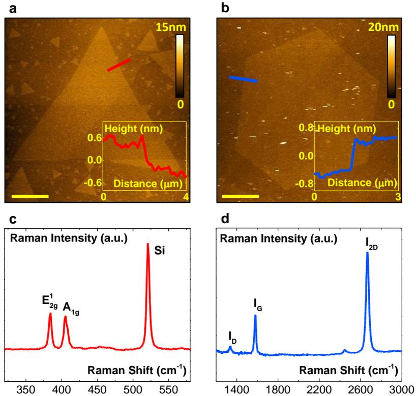
**Figure 12. Characterization of MoS<sub>2</sub> and Graphene Flakes.** (a-b) AFM topography maps of the direct-grown MoS<sub>2</sub> and transferred graphene flakes on Si/SiO<sub>2</sub> substrate. The scale bars are 5  $\mu$ m. (c-d) Raman point spectra obtained from the synthesized MoS<sub>2</sub> (c) and graphene (d) flakes.
