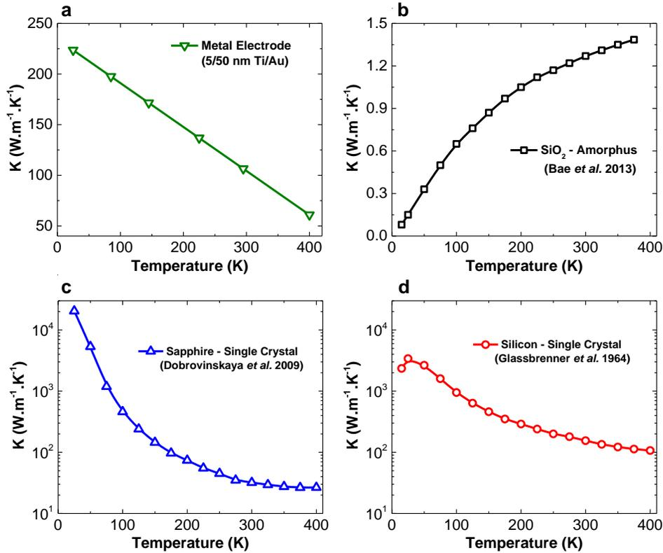
**Figure 16. Thermal Conductivities of The Materials vs. Temperature.** (a) Metal electrode through Wiedemann-Franz law[32], [216], (b) Silicon oxide ( $\text{SiO}_2$ ), (c) Sapphire single crystal, (d) Silicon single crystal.
