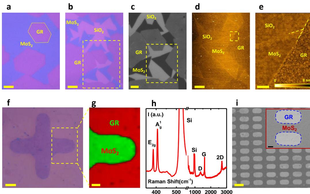
**Figure 27. Microscopy and Characterization of MoS<sub>2</sub>-Graphene In-Plane Heterostructure.**
