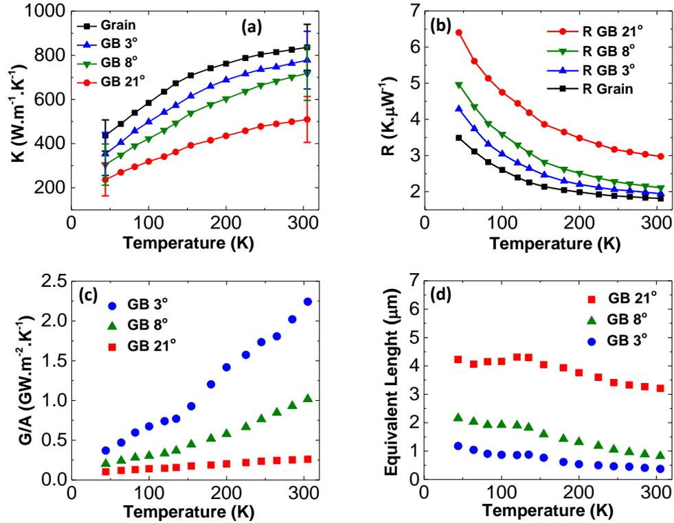
**Figure 10. Extraction and Analysis of the Experimental Data.** (a) Temperature-dependent extracted thermal conductivity of the single crystalline graphene and the GB region with different mismatch angles (3, 8, and 21 degrees). The error bars represent the overall uncertainty of the
