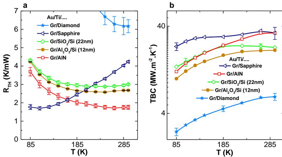
**Figure 23. Thermometry Results of Graphene Stacks on Silicon Substrate with Thin Oxides.** (a) R<sub>TH</sub> and (b) TBC versus Temperature results of Au/Ti/Gr/SiO<sub>2</sub>/Si (22nm) and Au/Ti/Gr/Al<sub>2</sub>O<sub>3</sub>/Si (12nm) stacks along with the graphene stack results on sapphire, AlN, and diamond substrates. The error bars in (a) indicate the standard deviation of >3 experiments in identical conditions. The error bars in (b) shows the uncertainty of the extracted TBC values.
