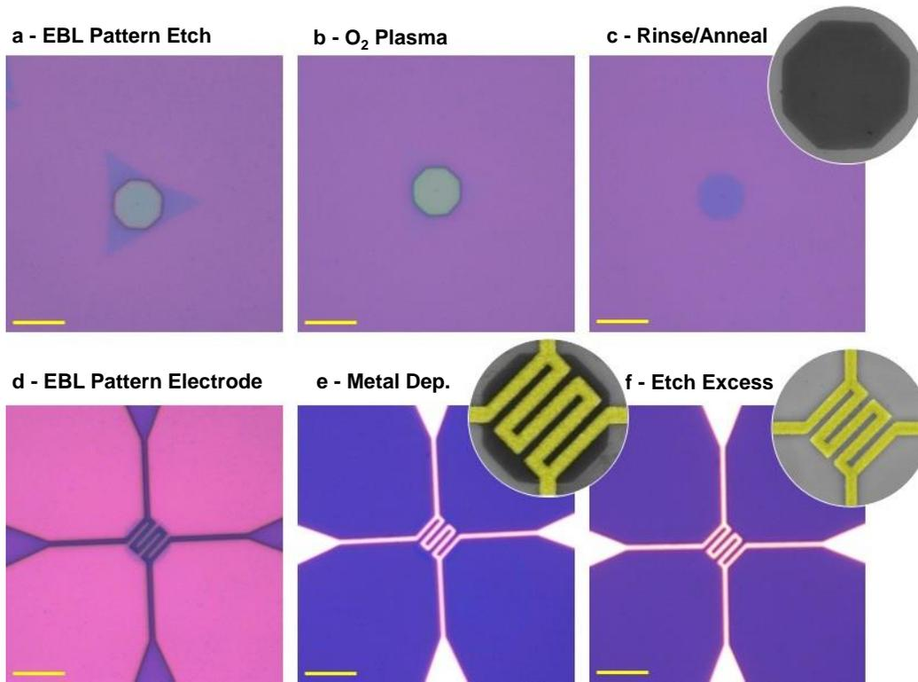
**Figure 13.** Different Steps of The Fabrication Process. The scale bars are 10  $\mu\text{m}$ .
