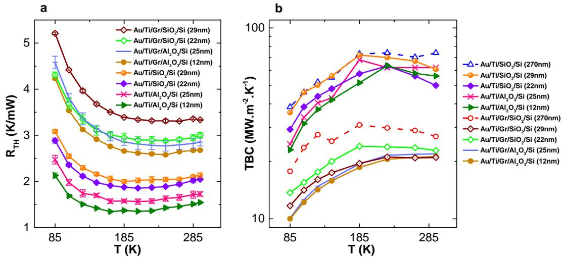
**Figure 24. The Full Dataset for The Thermometry Results on Silicon Substrate with Thin Oxides.** (a)  $R_{TH}$  and (b) TBC for different test structures on thin oxides at the temperature range of 85-295K. The TBC curves are plotted against the data for Si/SiO<sub>2</sub> (270nm) for comparison.
