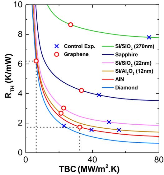
**Figure 25. Dependence of  $R_{TH}$  on TBC for All The Tested Structures.** The solid lines show the trends obtained from FE analyses and the symbols represent the experimental data. The dashed lines compare the  $R_{TH}$  and TBC between the Au/Ti/Gr/Diamond and Au/Ti/Gr/AlN stacks.
