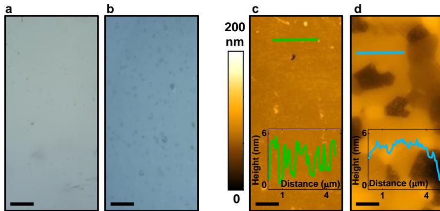
**Figure 19. Morphological Characterization of Diamond and AlN Substrates.** (a-b) Optical image of an as-received diamond and AlN substrates, respectively. The scale bars are 15  $\mu$ m. (c-d) AFM images of the diamond and AlN substrates, respectively. The scale bars are 2  $\mu$ m. The inset shows the height profile along the green and blue lines.
