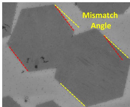
**Figure 3. Estimating the Crystallographic Mismatch Angle from Morphology.** SEM image of two merged hexagonally shaped single crystalline graphene grains forming an individual GB. The comparison of the edge orientations is used to estimate the crystallographic mismatch angle across the GB. The scale bar is 5  $\mu\text{m}$ .
