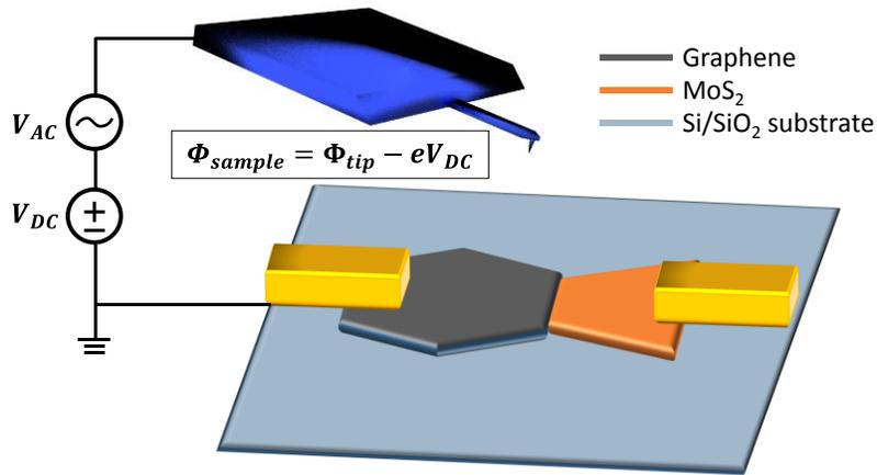
**Figure 32.** Schematic of Kelvin Probe Force Microscopy (KPFM) Setup.
