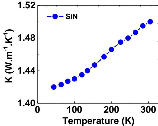
**Figure 9.** Extracted Thermal Conductivity of The SiN Membrane.
