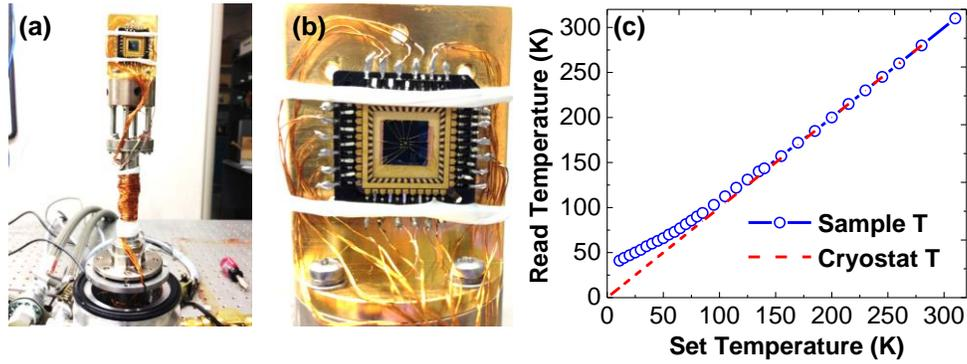
**Figure 6. Details of Experimental Setup** (a-b) Optical images of the measurement setup (c) Measured temperature drift between the sample and cold finger.
