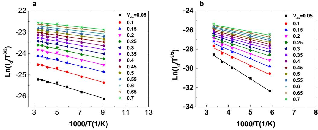
**Figure 29. Arrhenius Measurements at  $V_g=40V$  for Different Applied  $V_{ds}$  for (a),  $MoS_2/Gr$  (b),  $MoS_2/Metal$  transistors**
