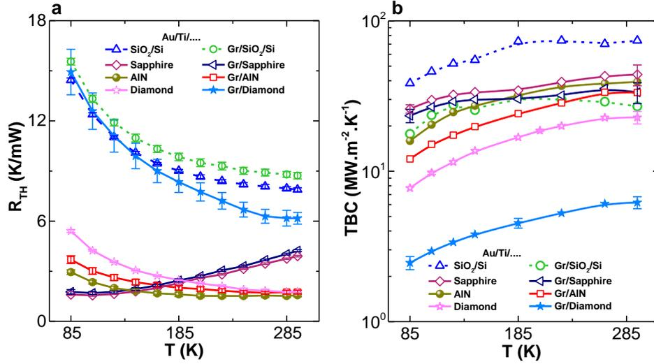
**Figure 21.** Full Dataset for (a)  $R_{TH}$  and (b) TBC for the Diamond, Sapphire, AlN, and Si/SiO<sub>2</sub> (270nm) Substrates.
