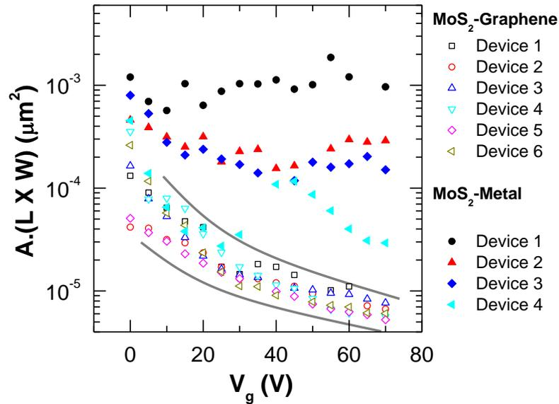
**Figure 34. Comparison of Area-Normalized Noise Amplitude of MoS<sub>2</sub>-Graphene and MoS<sub>2</sub>-Metal FETs as a Function of  $V_g$ .** Two gray lines show upper and lower bounds of noise amplitude for MoS<sub>2</sub>-graphene devices.
