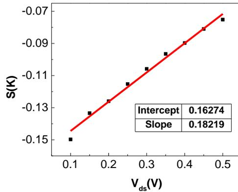
**Figure 30. Slope of the Arrhenius graph as a function of the  $V_{ds}$  at gate 40 V.**
