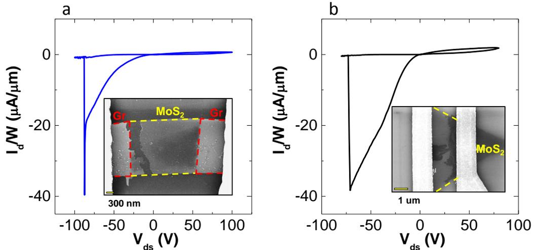
**Figure 35. Breakdown Study of MoS<sub>2</sub>-Graphene and MoS<sub>2</sub>-Metal FETs.** (a), (b) Current-voltage characteristics of a MoS<sub>2</sub>-graphene and MoS<sub>2</sub>-metal FET, respectively, at  $V_g = 0$  V showing irreversible breakdown at large  $V_d$ . The current was normalized to the channel width. The insets of (a) and (b) show scanning electron microscopy micrographs of the MoS<sub>2</sub>-graphene and MoS<sub>2</sub>-metal FETs after the breakdown, respectively.
