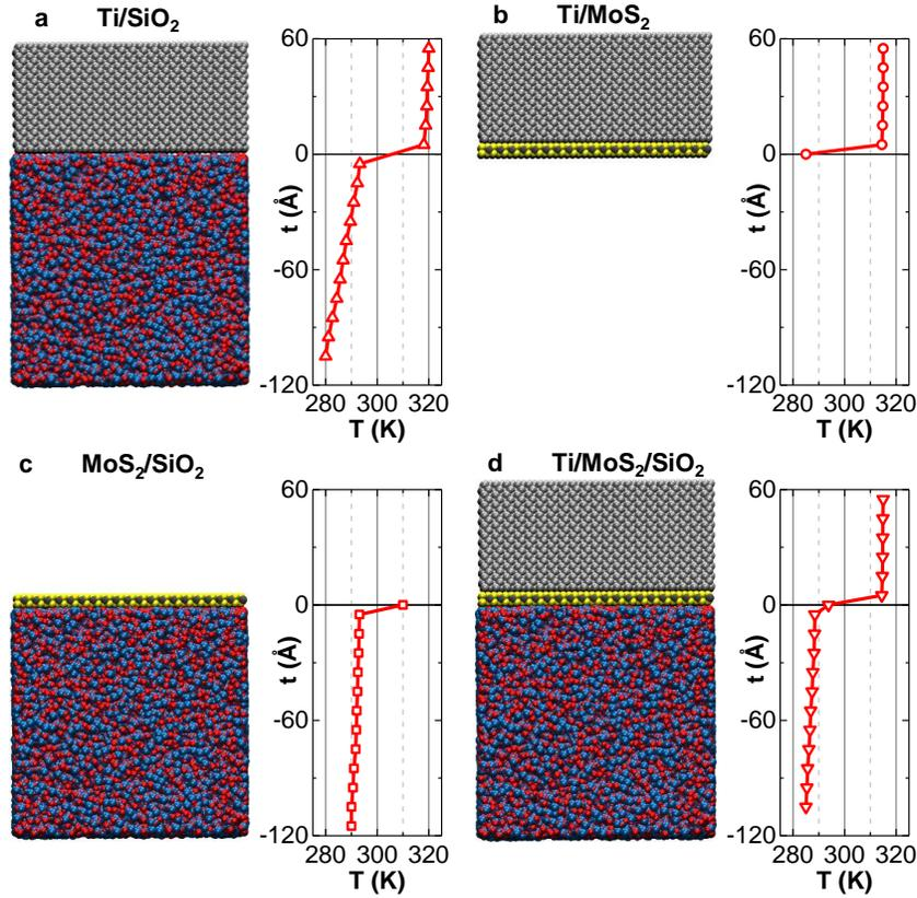
**Figure 18. Snapshots of The Four MD Simulation Systems Consisting of Ti, MoS<sub>2</sub>, and SiO<sub>2</sub>.** For each system, the temperature profile normal to the plane of MoS<sub>2</sub> obtained from the NEMD simulations is shown. The temperature profiles are used to calculate the TBC at each boundary.
