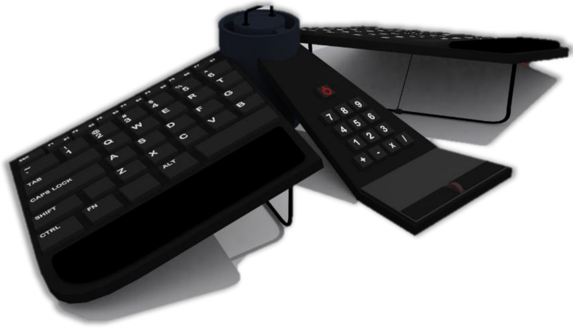
Figure 11: Trinity keyboard design in the tented position displaying its tilting feature
