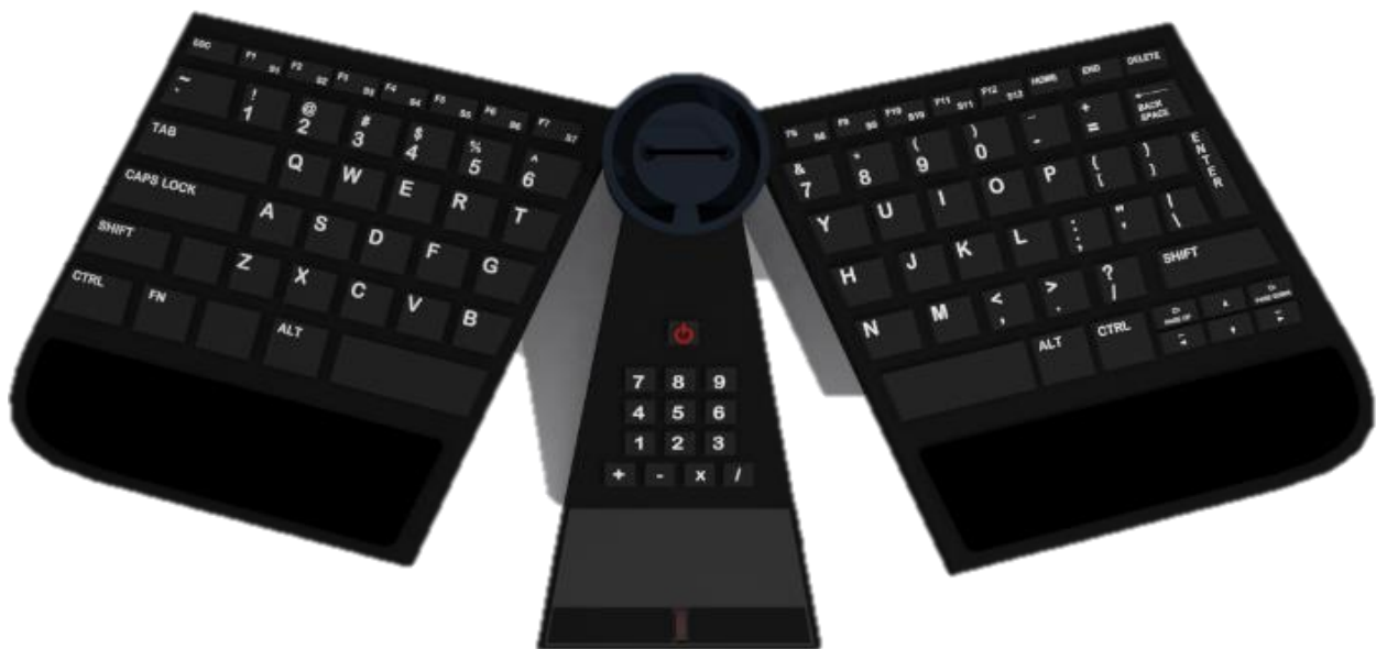
Figure 9: Trinity gull-wing position; the keyboard is split in three parts at favorable angles
