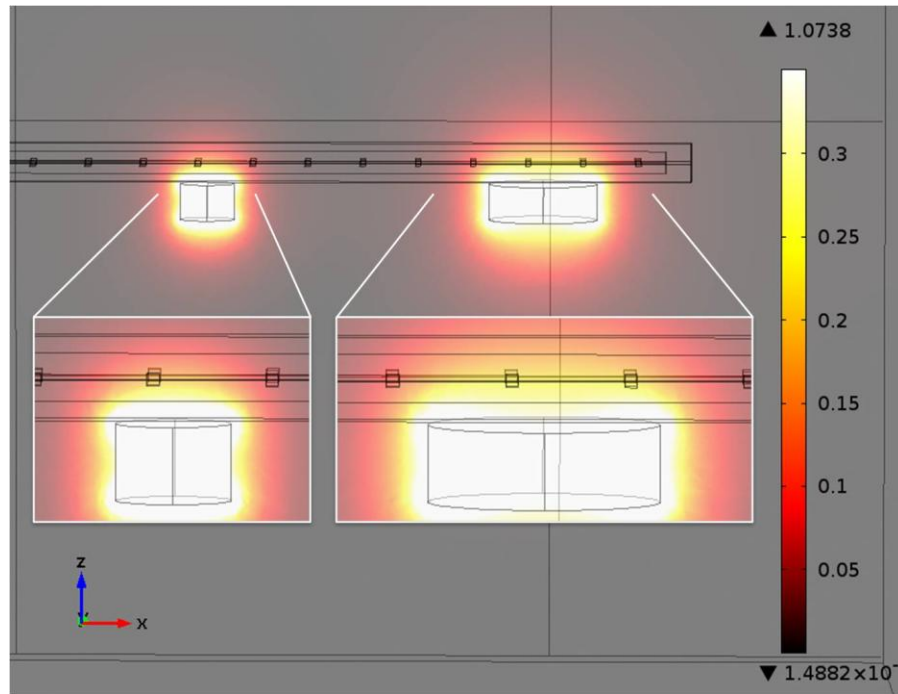
Figure 33. Magnetic field produced by targeting magnet and barrier magnet (shown in xz-plane). CSF-filled subarachnoid space opposite the targeting magnet experiences a magnetic field \vec{B} in the range of 0.051-0.098 T (510-980 gauss), while the subarachnoid space opposite the barrier magnet experiences a \vec{B} field in the range of 0.092-0.167 T (920-1670 gauss). Figure inserts are close-up views of both magnets to show more detail.
