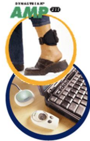
Figure 5-4: AMP activity monitor placement (top) and data transfer setup (bottom).
