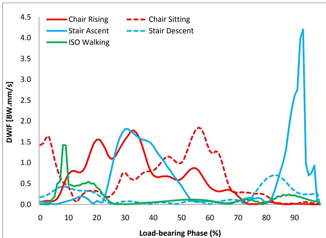
Figure 6-16: Directional wear index factor for chair, stair and ISO walking throughout the load-bearing cycle. The spike exhibited by stair ascent at about 90% of the load-bearing cycle, was caused by the coincidence of the peak load and a high rotational value generated during stair ascent.
