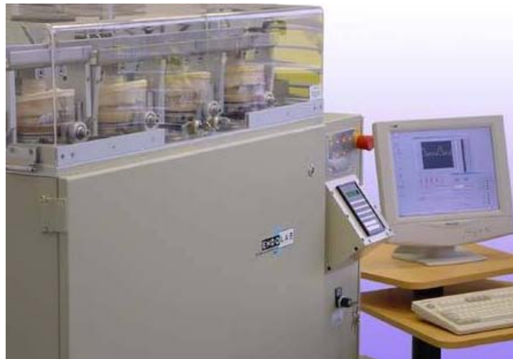
Figure 6-2: EndoLab (Rosenheim, Germany) four-station knee simulator. Lubricant in the test stations for this study was distilled water.
