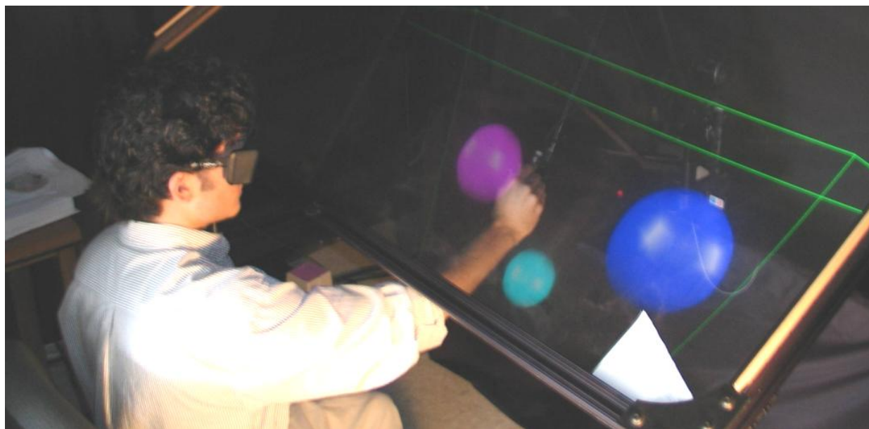
Figure 1- Components of the VRRROOM apparatus. Large virtual spheres rendered both haptically by the robot and graphically by the PARIS display. Magnetic tracking sensors detect head position in space.
