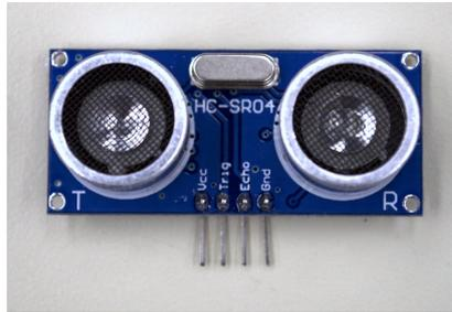
Figure 13: The HCSR04 ultrasound sensor.
