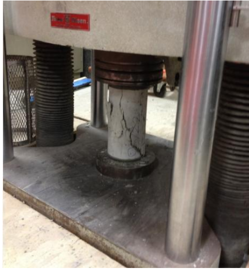
Figure 3.2. Compressive Strength Test (ASTM C39)
