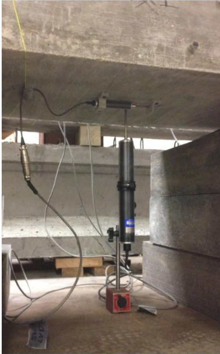
Figure 3.24. Vertical LVDT for Deflection Measurement and Horizontal LVDT to Measure the Tensile Strain in Concrete
