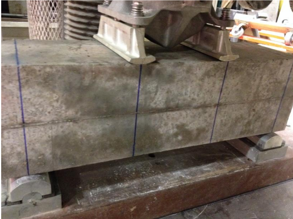
Figure 3.4. Flexural Strength Test of Concrete Beams (ASTM C78)
