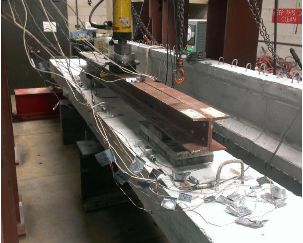
Figure 3.20. Laboratory Setup for Testing Continuous Slabs CS1 and CS2
