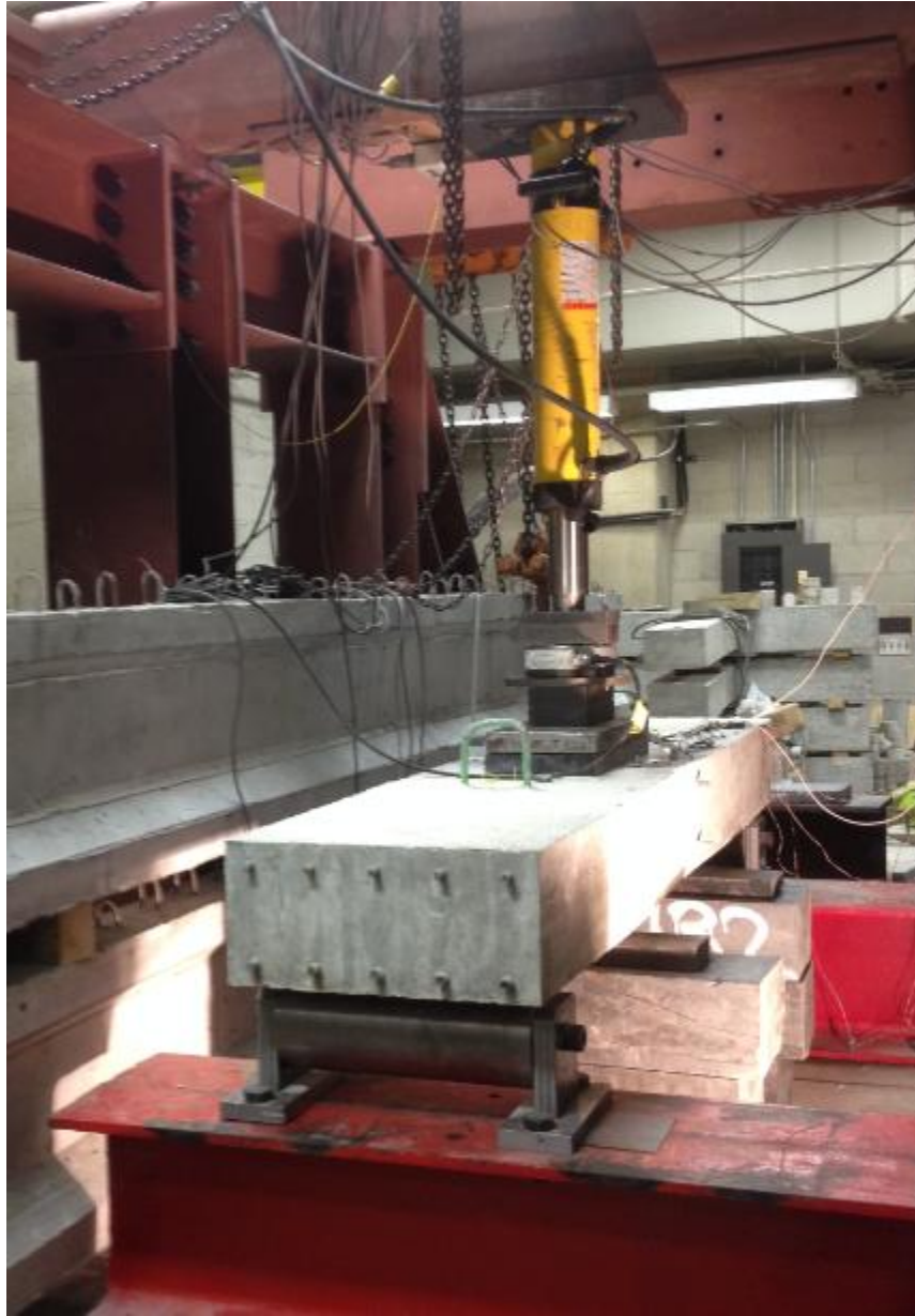
Figure 3.15. Laboratory Setup for Simply Supported Slabs
