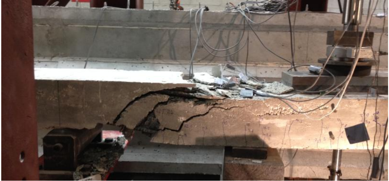
Figure 4.11. Shear Failure of Specimen SS3-CS1
