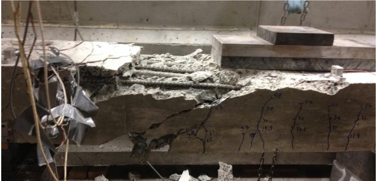
Figure 4.27. Flexural Shear Failure of Specimen CS2
