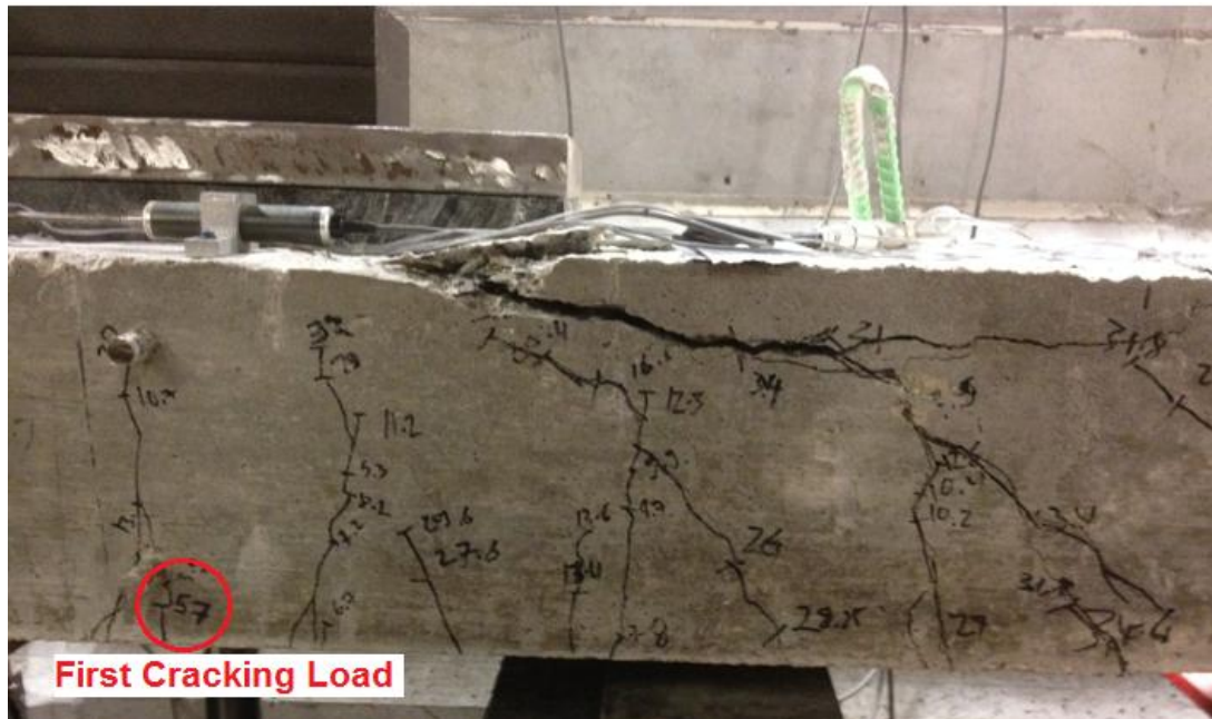
Figure 4.2. (a) Flexural Shear Failure of Specimen SS2
