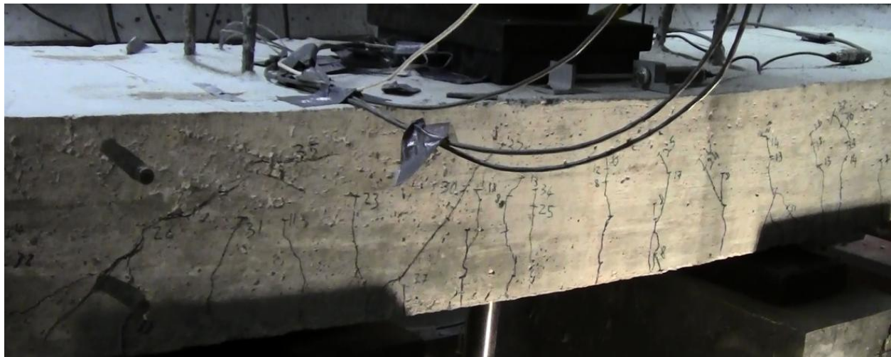
Figure 4.37. Left Span Cracking and Deflection of Slab CS1
