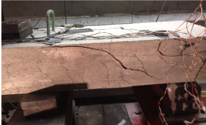
Figure 4.1. Flexural Shear Failure of Specimen SS1
