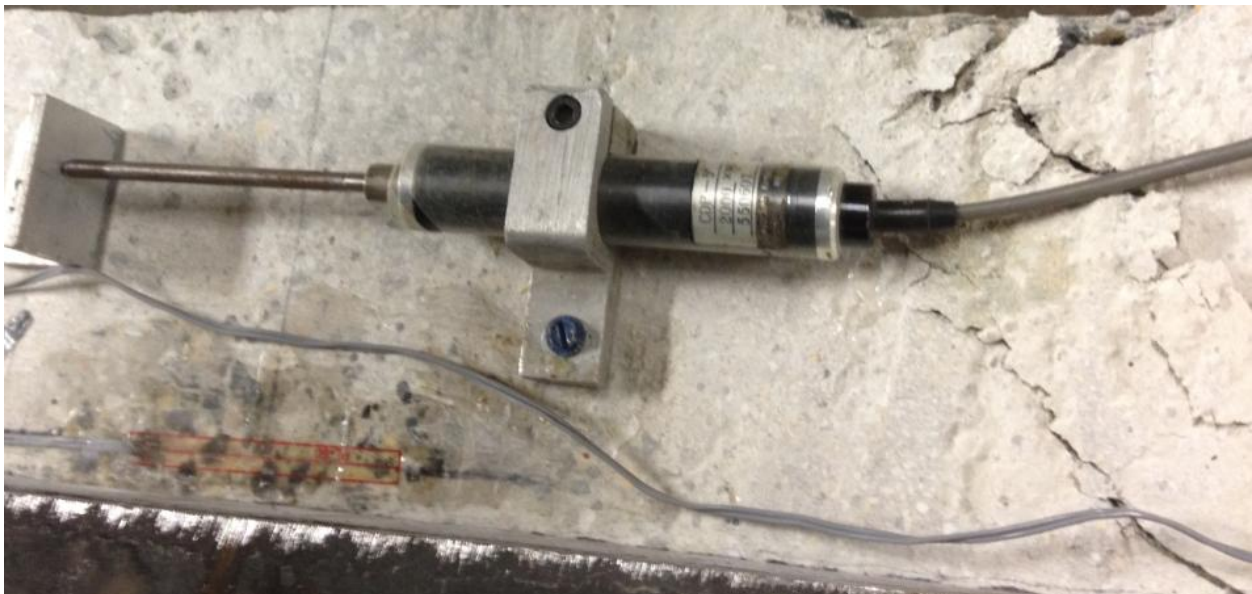
Figure 3.23. Strain Gage and Horizontal LVDT to Measure the Compressive Strain in Concrete
