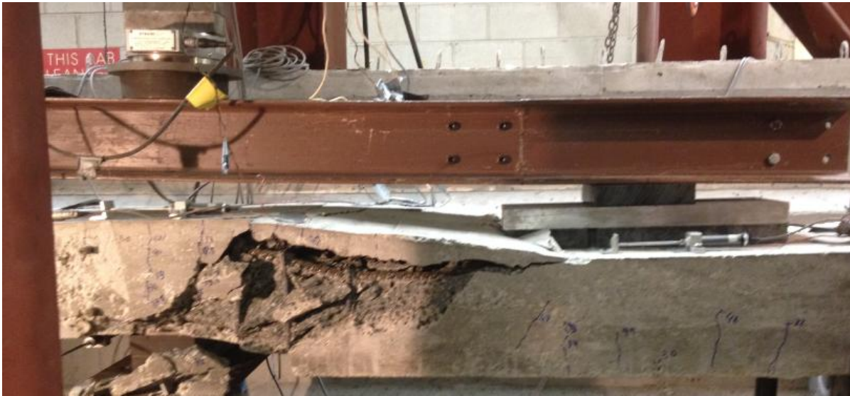
Figure 4.26. Flexural Shear Failure of Specimen CS1
