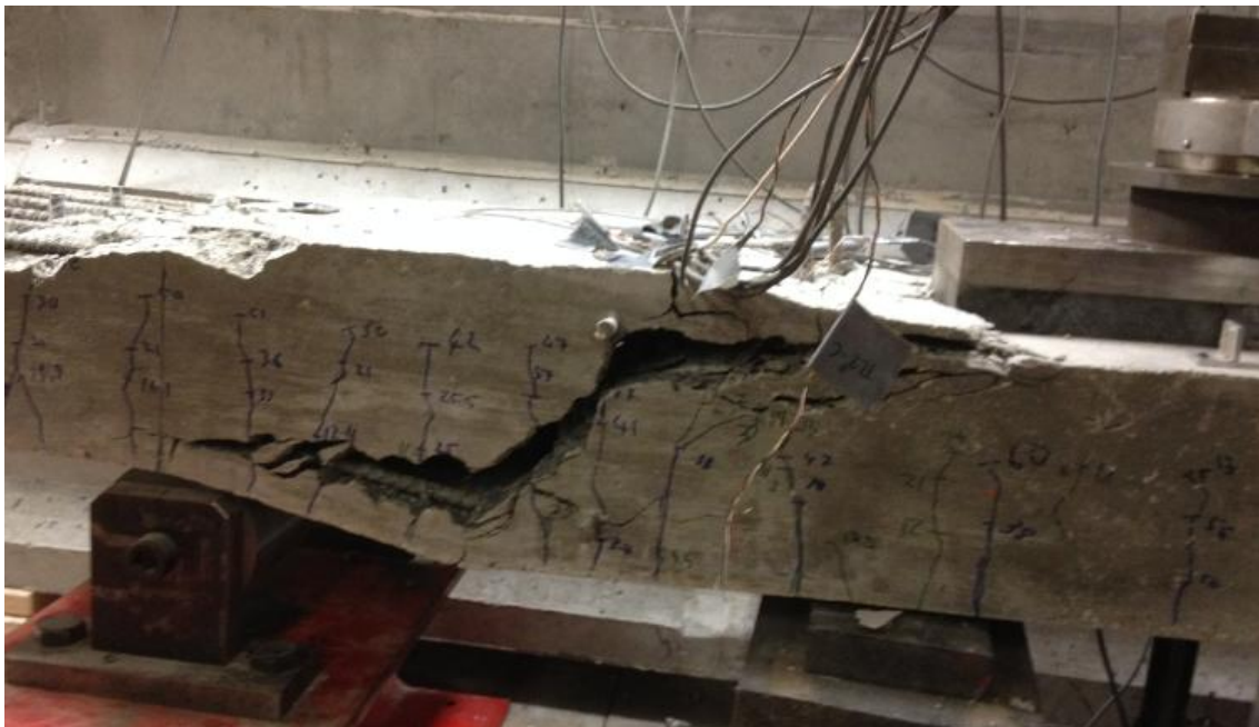
Figure 4.19. Shear Failure of Specimen SS6-CS2
