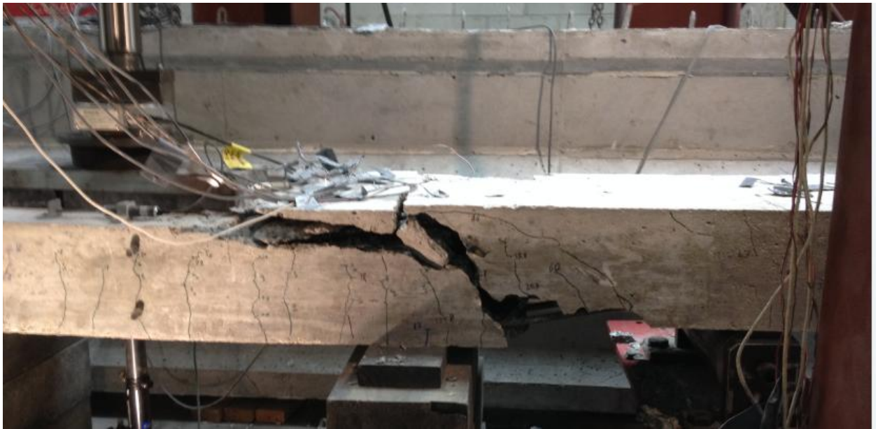
Figure 4.12. Shear Failure of Specimen SS4-CS2
