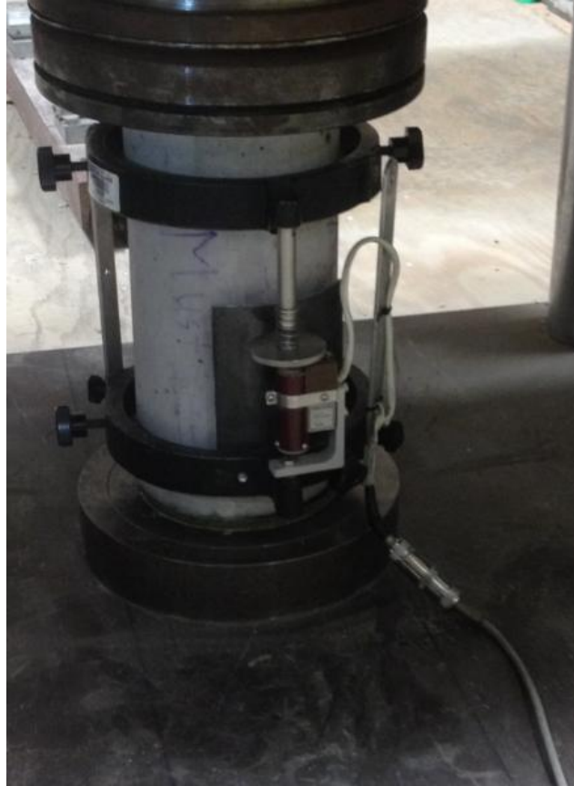
Figure 3.5. Modulus of Elasticity Test Fixture - ASTM C469
