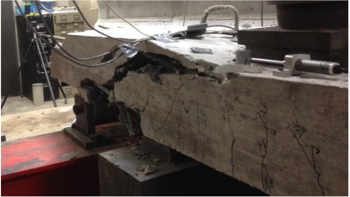
Figure 4.18. Shear Failure of Specimen SS5-CS1
