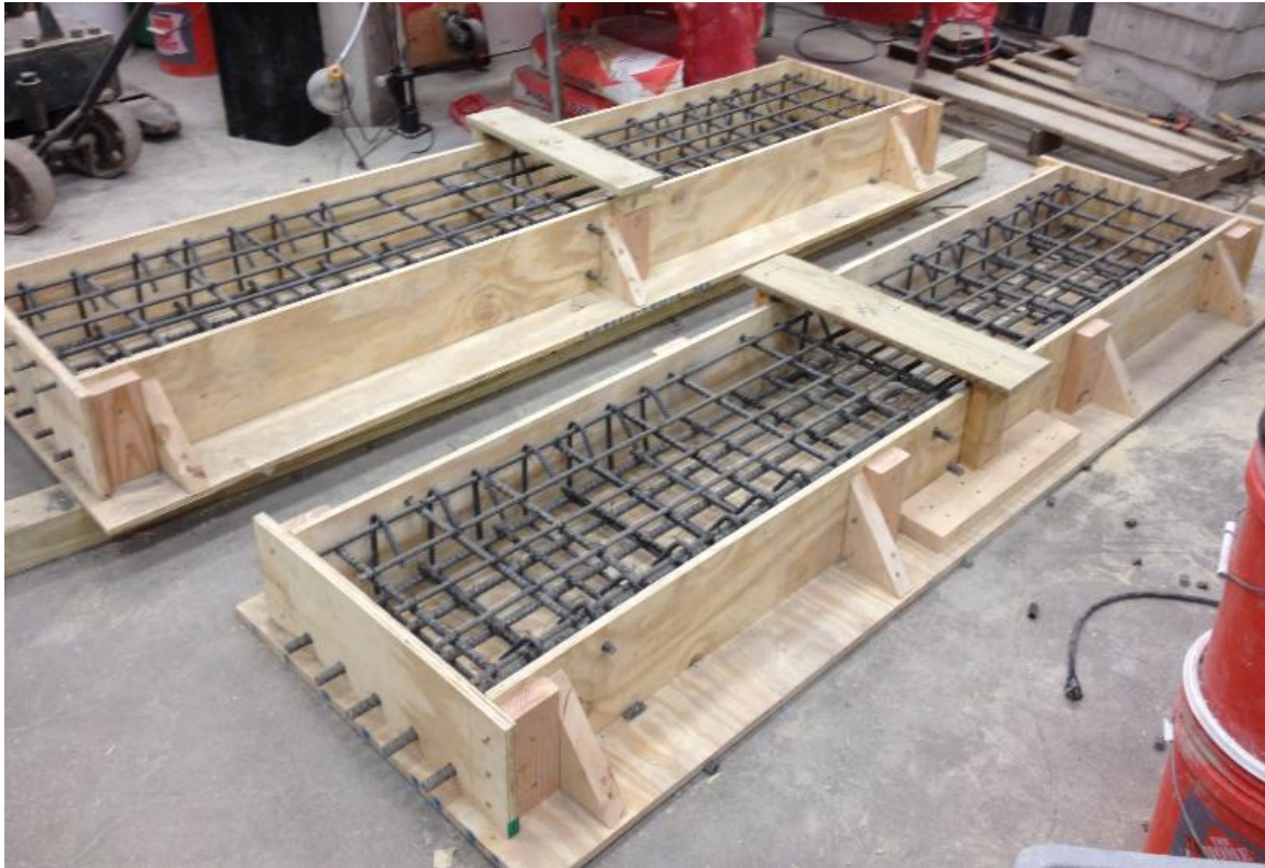
Figure 3.7. Finalized Formworks for Simply Supported Specimens SS1 and SS2
