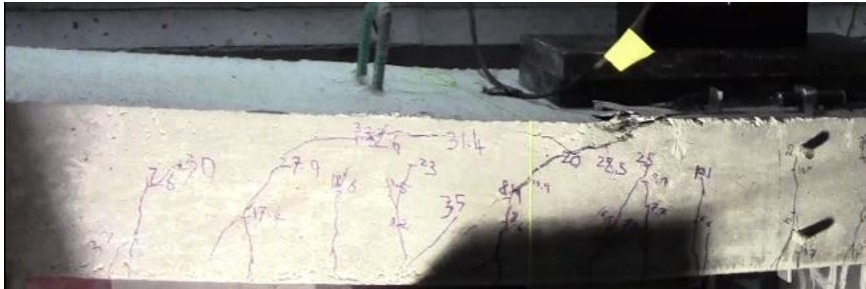
Figure 4.36. Deflected Shape and Cracks for Slab SS2
