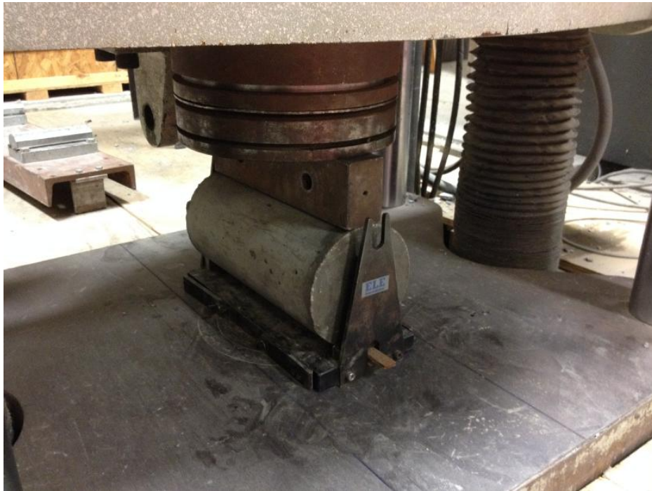
Figure 3.3. Splitting Tensile Strength Test (ASTM C496)
