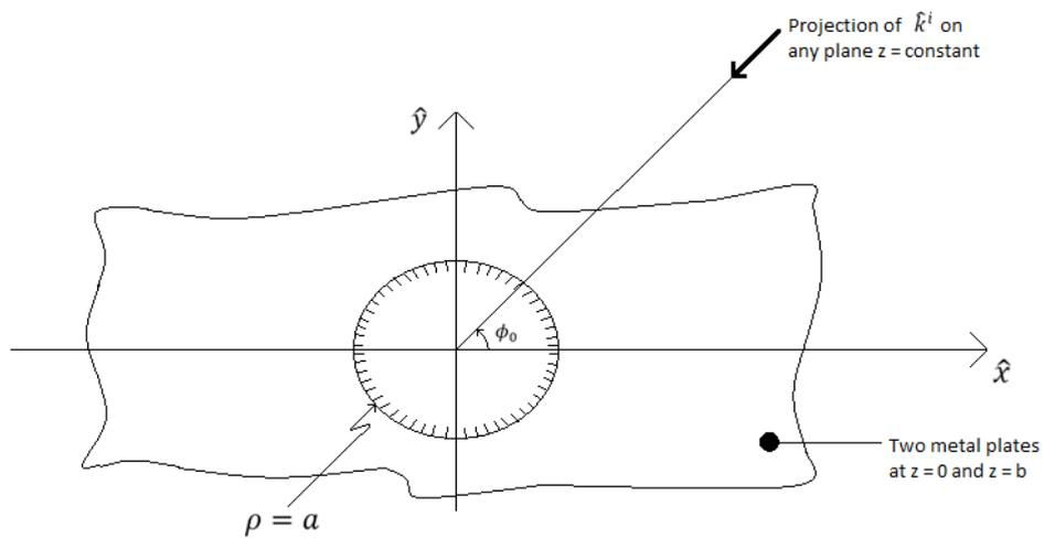
Figure 5: Top view of a circular-cylinder post inside a parallel plate waveguide
