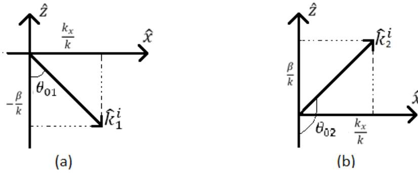
Figure 3: Two incident plane waves, (a) Plane wave 1 is propagating in the direction  $\hat{k}_1^i$  and makes an angle  $\theta_{01}$  with the negative z-axis. (b) Plane wave 2 is propagating in the direction  $\hat{k}_2^i$  and makes an angle  $\theta_{02}$  with the negative z-axis.
