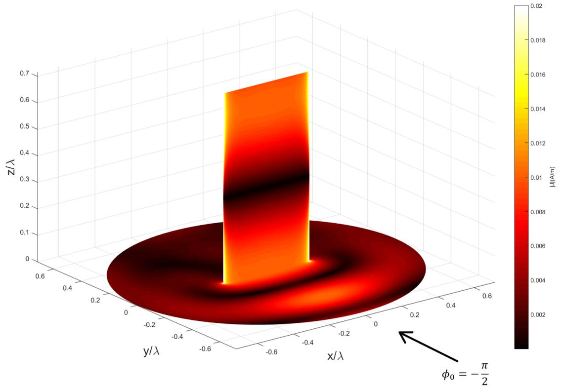
Figure 12:  $|J_{u/z}|$  on PEC Surfaces in case of metal strip post (E-polarization)
