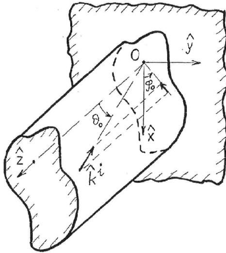
Figure 1: Plane wave incident on a cylinder truncated by a flat surface
