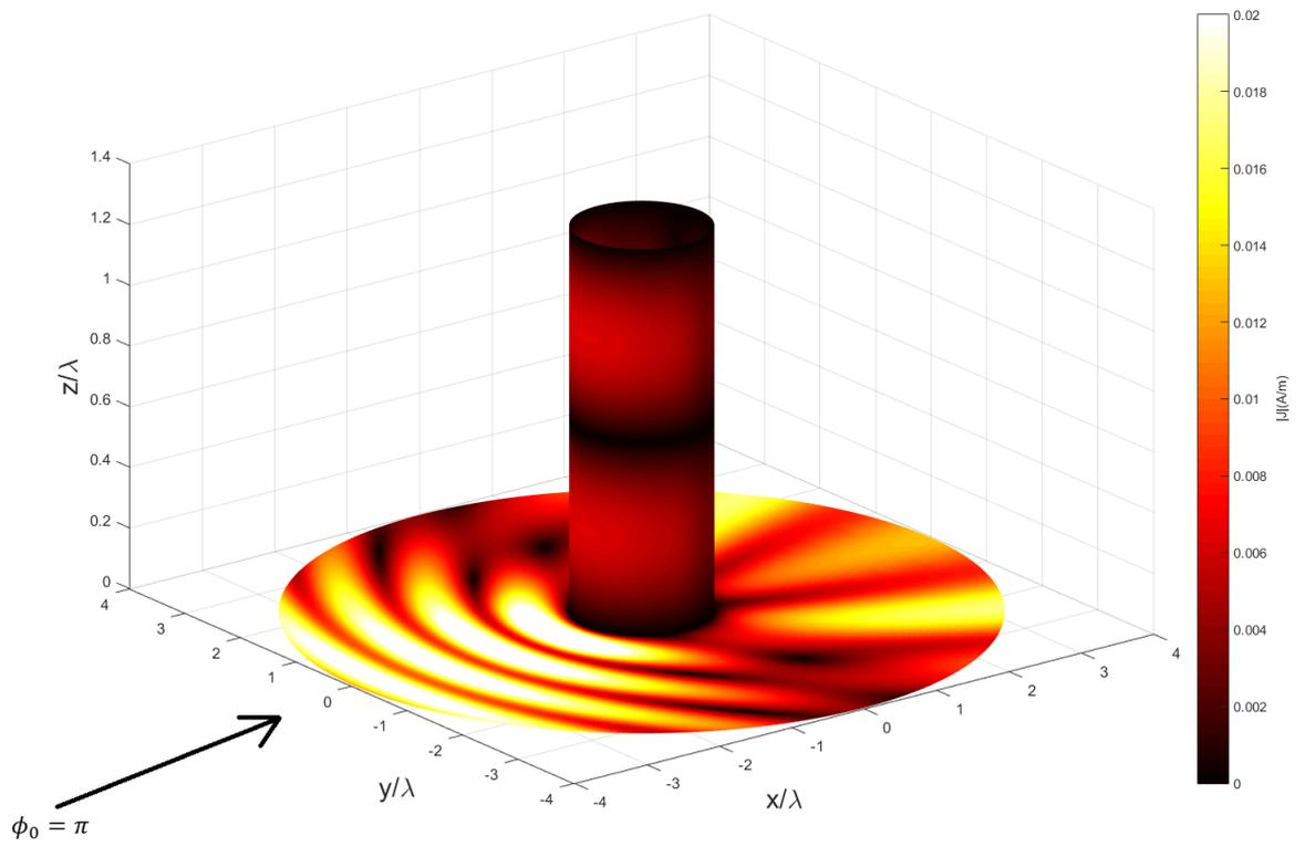
Figure 11:  $|J_\phi|$  on PEC Surfaces in case of cylindrical post (H-polarization)
