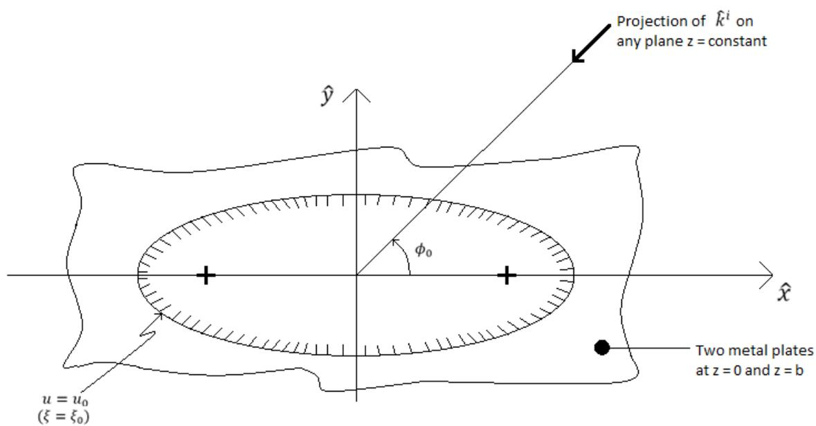
Figure 6: Top view of an elliptic-cylinder post inside a parallel plate waveguide
