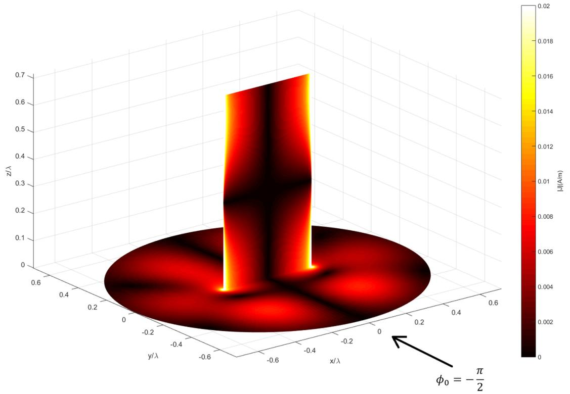
Figure 14:  $|J_{u/z}|$  on PEC Surfaces in case of metal strip post (H-polarization)
