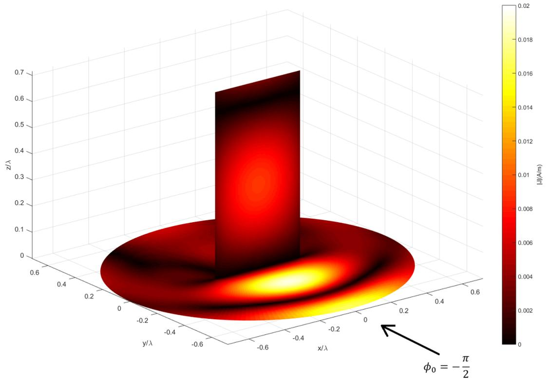
Figure 15:  $|J_v|$  on PEC Surfaces in case of metal strip post (H-polarization)
