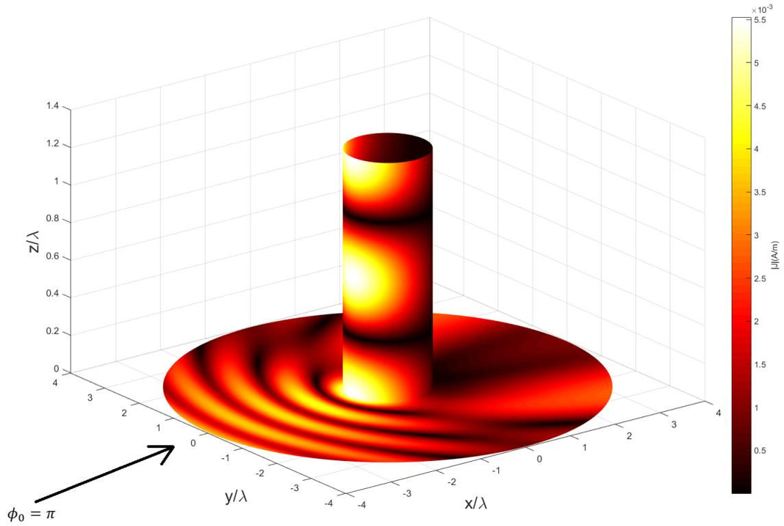
Figure 8:  $|J_{\rho/z}|$  on PEC Surfaces in case of cylindrical post (E-polarization)
