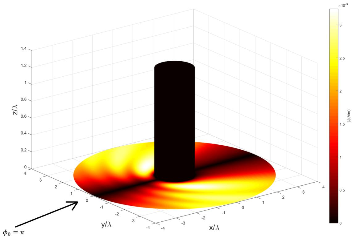
Figure 9:  $|J_\phi|$  on PEC Surfaces in case of cylindrical post (E-polarization)
