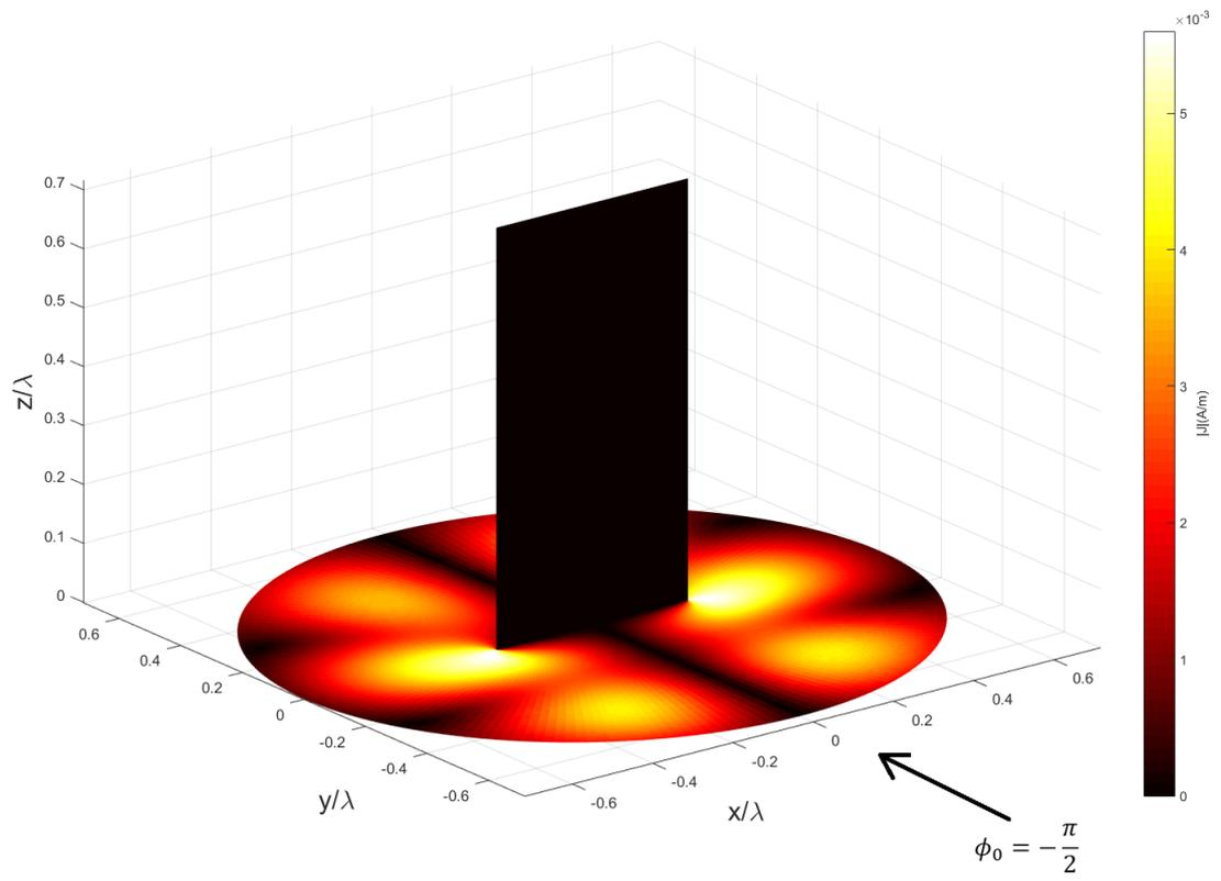
Figure 13:  $|J_v|$  on PEC Surfaces in case of metal strip post (E-polarization)
