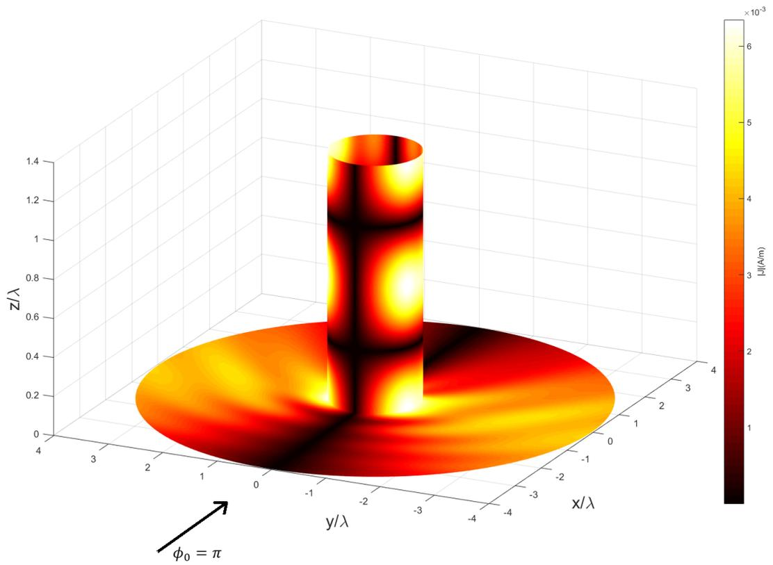
Figure 10:  $|J_{\rho/z}|$  on PEC Surfaces in case of cylindrical post (H-polarization)
