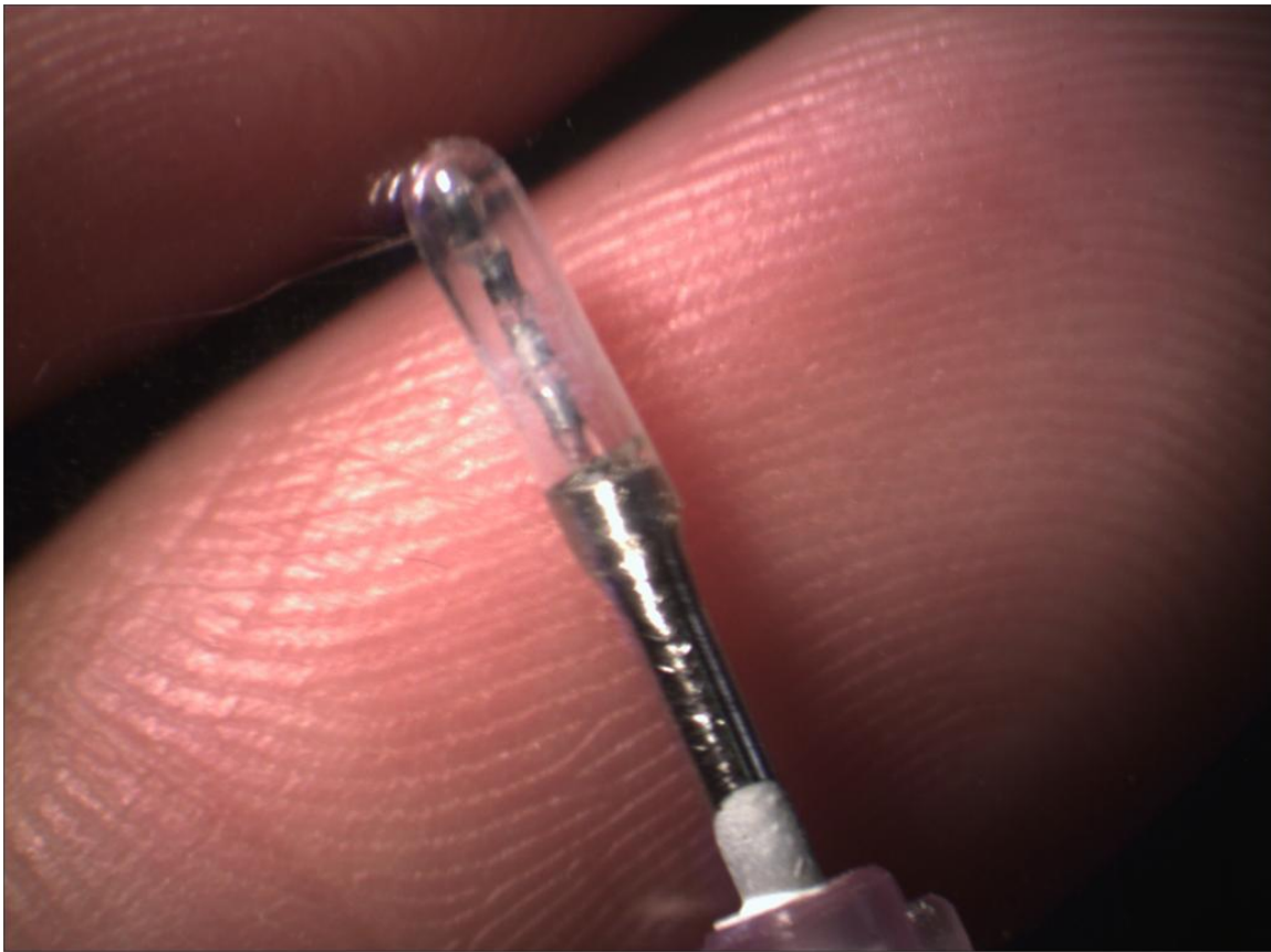
Figure 16. Completed Silicone Balloon Model. The sensor is visible inside.
