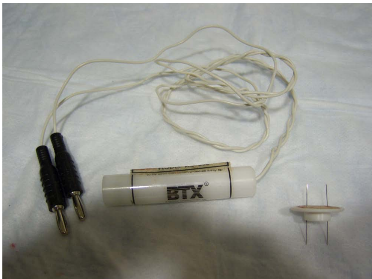
Figure 3.1: IRE electrodes and its holder
