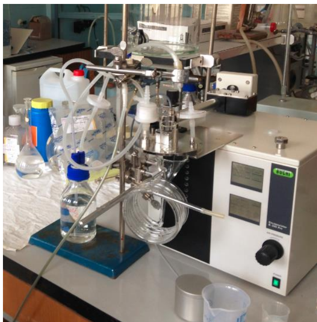
Figure 5-3: Buchi Encapsulator B395 Pro™ testing with PMCG polymer system.
