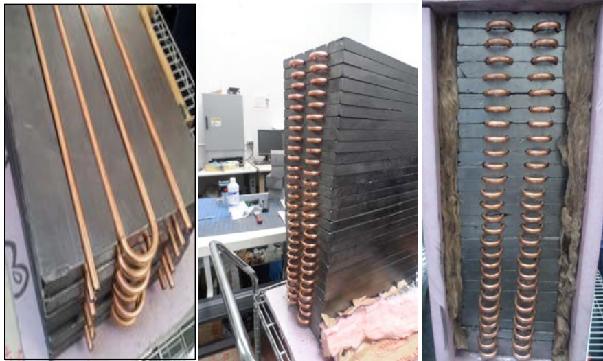
Figure 3b: Actual representation of the proposed PCC-TES system
