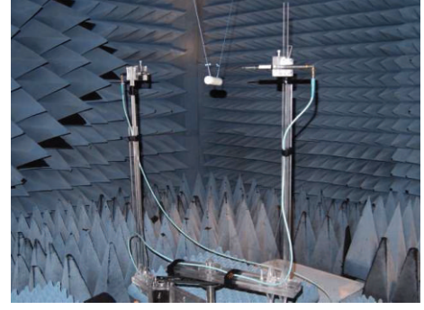
FIGURE 1: Experimental setup. The TX is on the left, the RX is on the right, and a target is visible in the top center, hanging from the ceiling.
