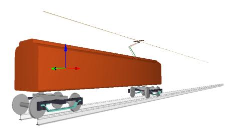
Figure 23: Pantograph/catenary railroad vehicle model
