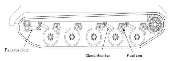
Figure 4: Suspension system layout of the tracked vehicle
