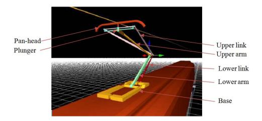
Figure 24: Articulated pantograph System
