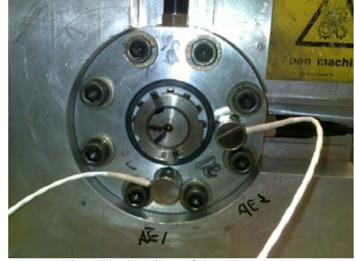
Fig. 5 The locations of the AE sensors.
