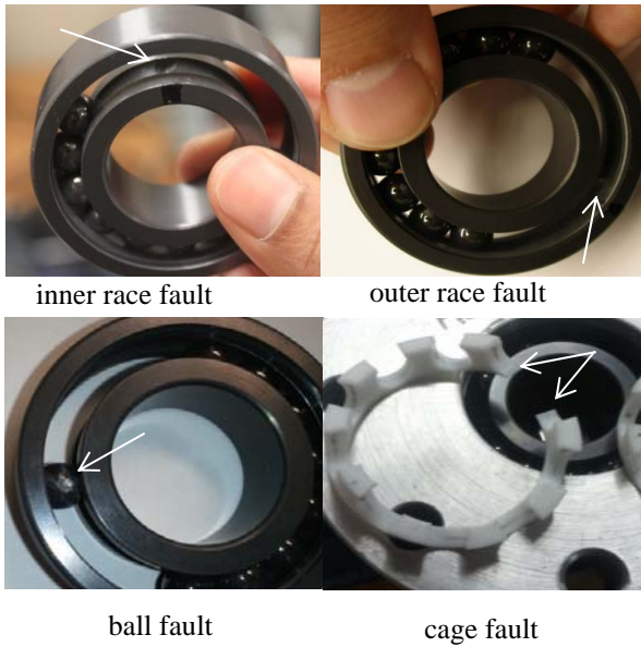
Fig. 4 The four bearing seeded faults.
