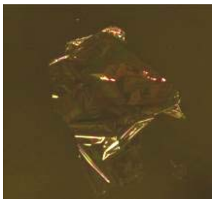
Figure 16. Transparent film formed after evaporating 0.1 g droplet of 5 wt% PAN solution in DMF.
