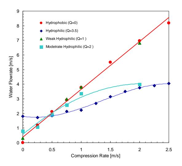
Figure 4. Flow velocity of water in nanochannels with hydrophobic and hydrophilic surfaces as a function of compression rate.
