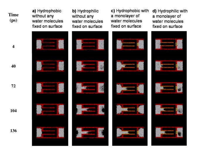
Figure 2. Capillary flow of water in nanochannels with hydrophobic (a) and hydrophilic (b) wall surfaces. To verify the effect of surface wettability on the water flow behavior, a monolayer of water molecules is fixed on both hydrophobic (c) and hydrophilic (d) surfaces for comparison.
