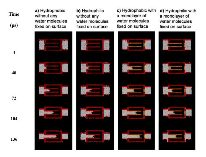
Figure 3. Forced flow of water in nanochannels with hydrophobic (a) and hydrophilic (b) wall surfaces. To verify the effect of surface wettability on the water flow behavior, a monolayer of water molecules is fixed on both hydrophobic (c) and hydrophilic (d) surfaces for comparison. The compression rate is 1.08 m/s.
