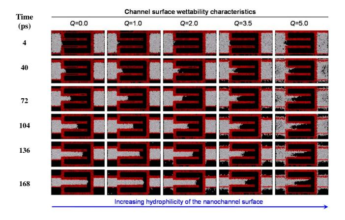
Figure 5. Effect of channel surface wettability on the forced flow rate of water in nanochannels. The compression rate is 1.08 m/s.
