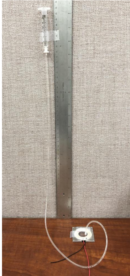
Figure B.4 Experimental setup used to determine the watertightness of DOMES.
