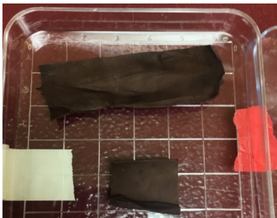
Figure 15: Carbonization - Fibers made by turbostratic graphite layers.
