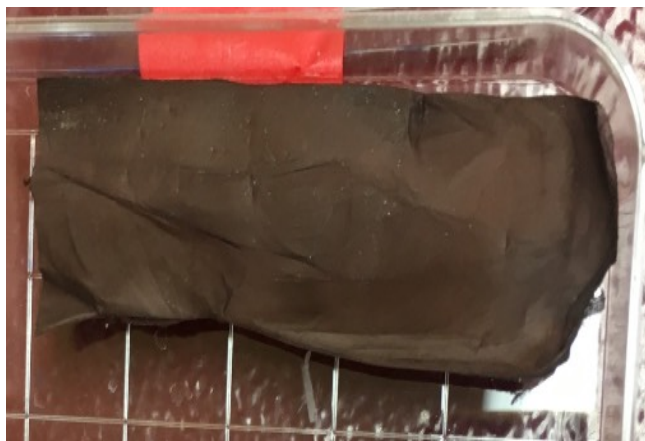
Figure 16: Turbostratic graphite fiber.
