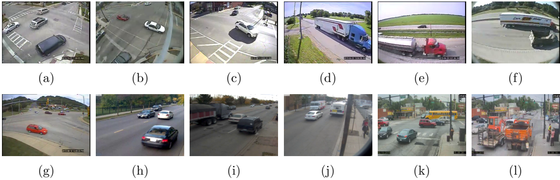
Figure 40: Snapshots of videos in our dataset, with various resolution, viewpoint, illumination, vehicle size and interactions. In particular, (c) shows shadows; (f) and (g) show severe distortion by fish-eye camera. We group these videos by their characteristics: (a) - (g) are simple low resolution videos (lowRes), and (h) - (l) are complex high resolution videos (highRes).
