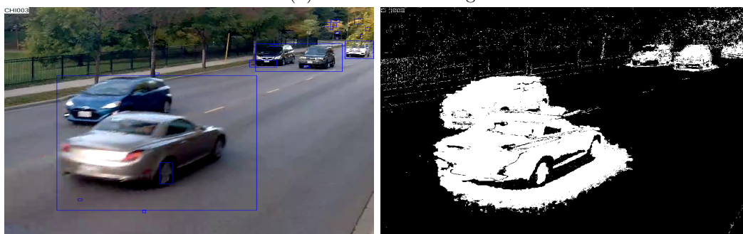
(c) Occlusion. Note also the shadow, due to illumination change.
