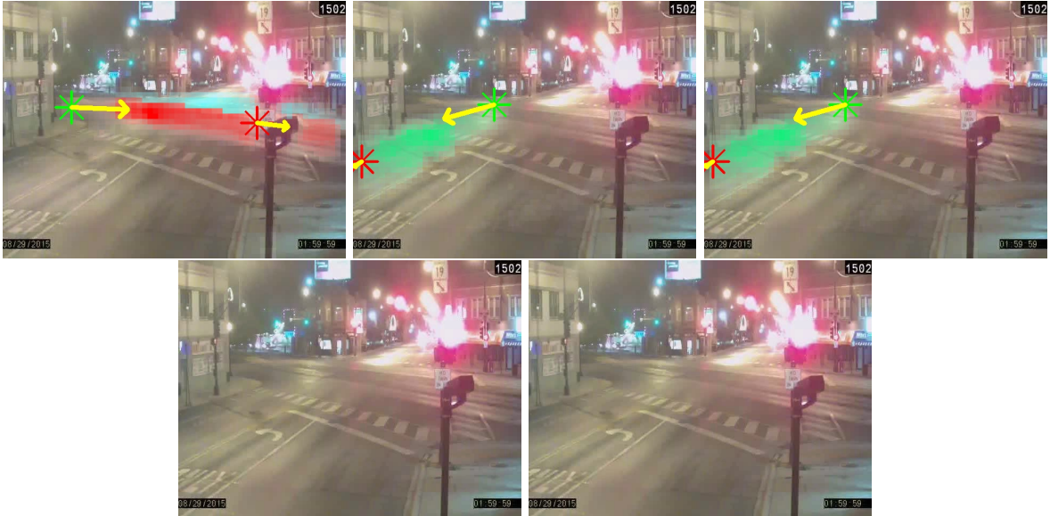
Figure 23: Model training on sparse night video about 5 minutes. Entry (green) and exit (red) locations with direction (yellow arrows).
