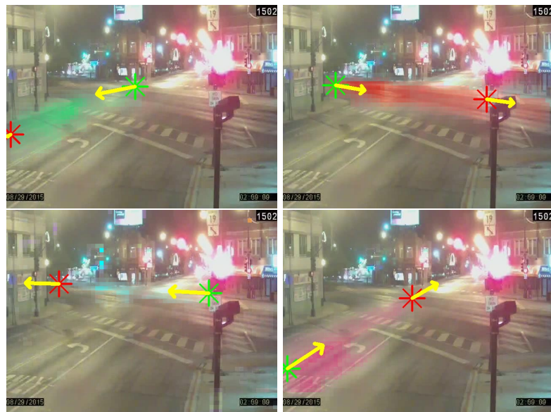
Figure 24: Model training on sparse night video about 30 minutes. Entry (green) and exit (red) locations with direction (yellow arrows).
