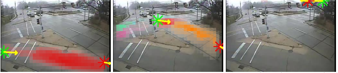
Figure 21: Failure case with simultaneous opposite directions. Entry (green) and exit (red) locations with direction (yellow arrows).
