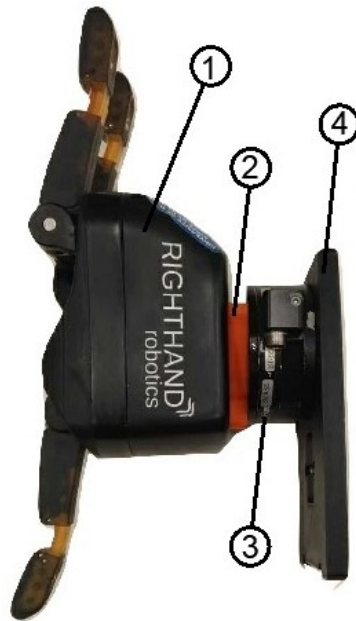
Figure 7: Complete mounting of the hand on the arm.
