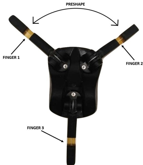
Figure 2: Reflex Sf with around 90^\circ of pre-shape angle.
