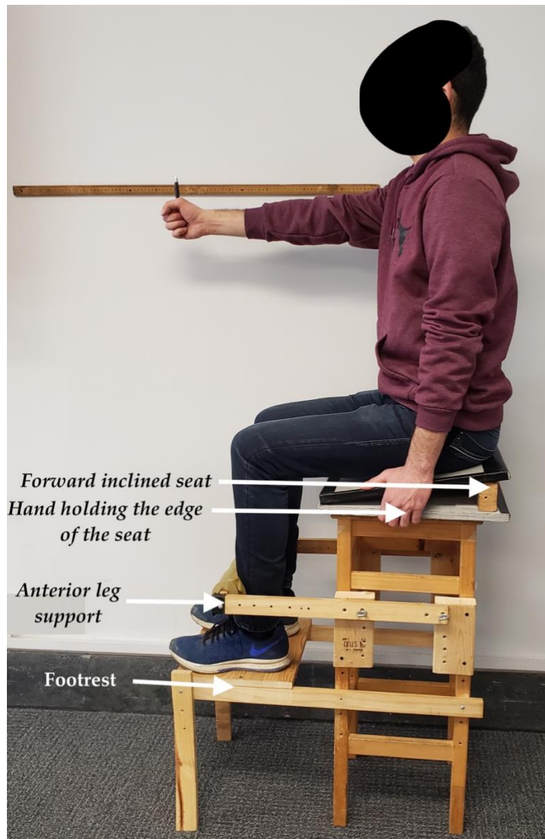
Fig. 3.1. Experimental setup showing different parts of the chair and body position.
