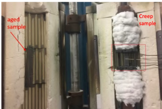
Figure 51. Locations of creep and aged sample inside the furnace for creep rupture test.
