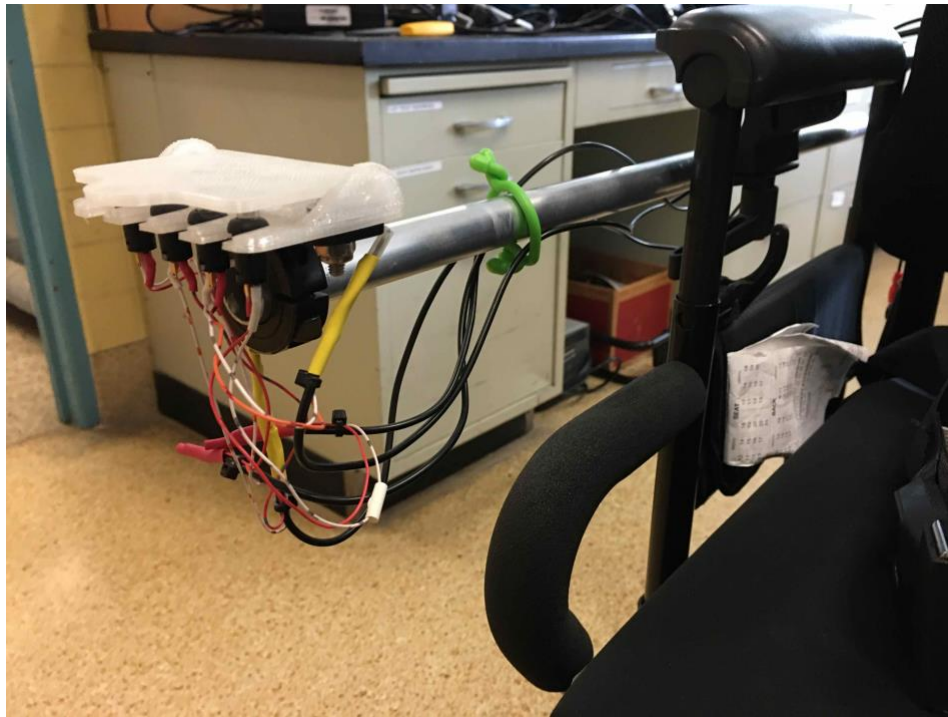
Figure 22. 3D-printed switch holder and activation lid.
