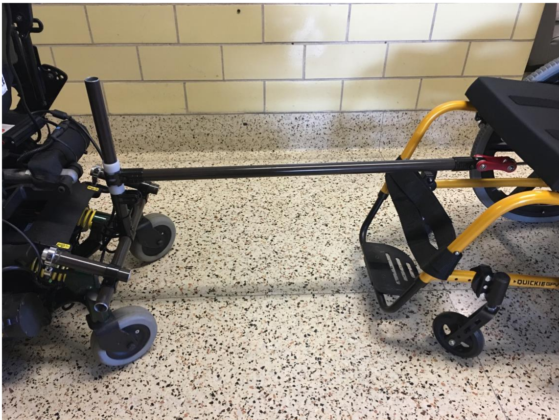
Figure 14. Custom tow bar between powered wheelchair and data collection manual wheelchair (Creform Material Handling Systems, Greer, SC).
