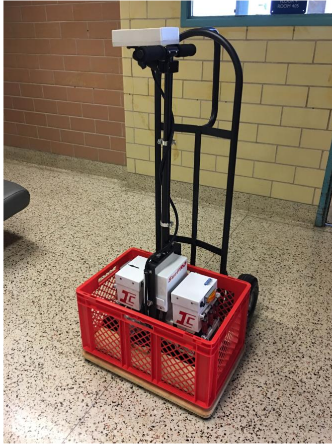
Figure 9. SurPRO 4000 in custom-fabricated cart, allowing transport to sites.
