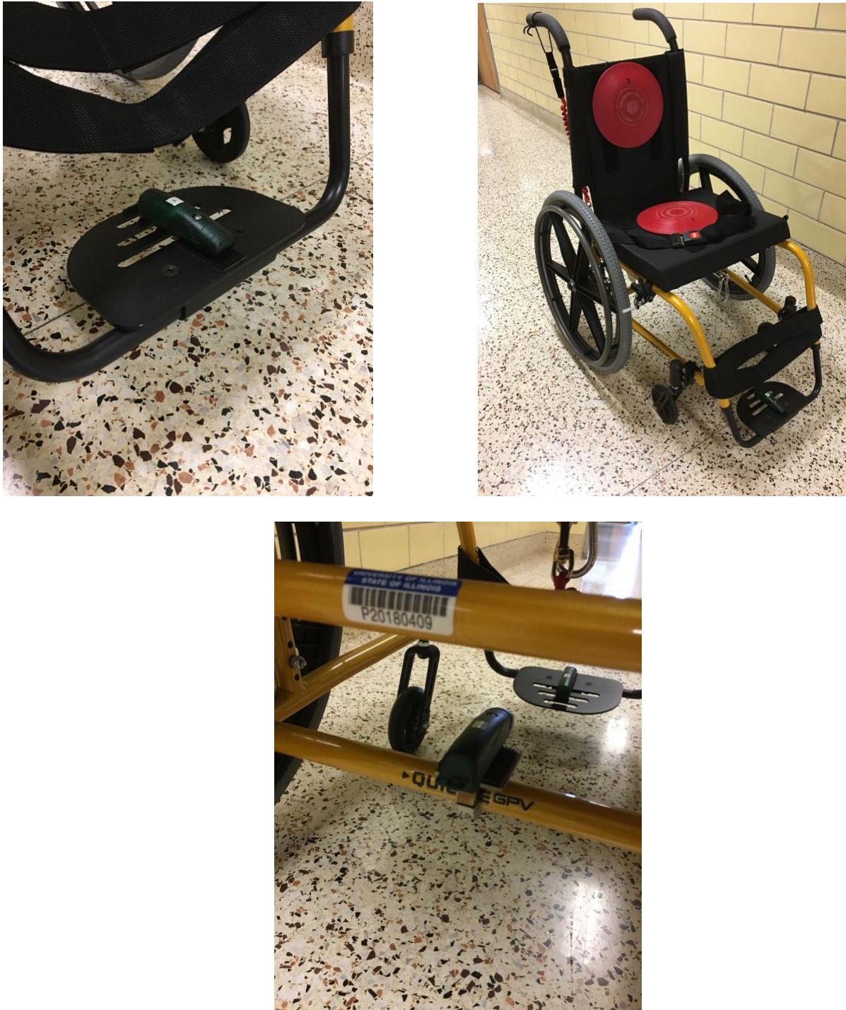
Figure 20. (a) A1 at footplate, (b) A2 at seat and A3 at backrest, (c) A4 at wheelchair frame cross member.
