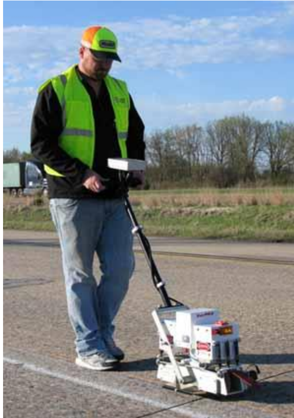
Figure 8. SurPRO 4000 device in use (International Cybernetics, Largo, FL).
