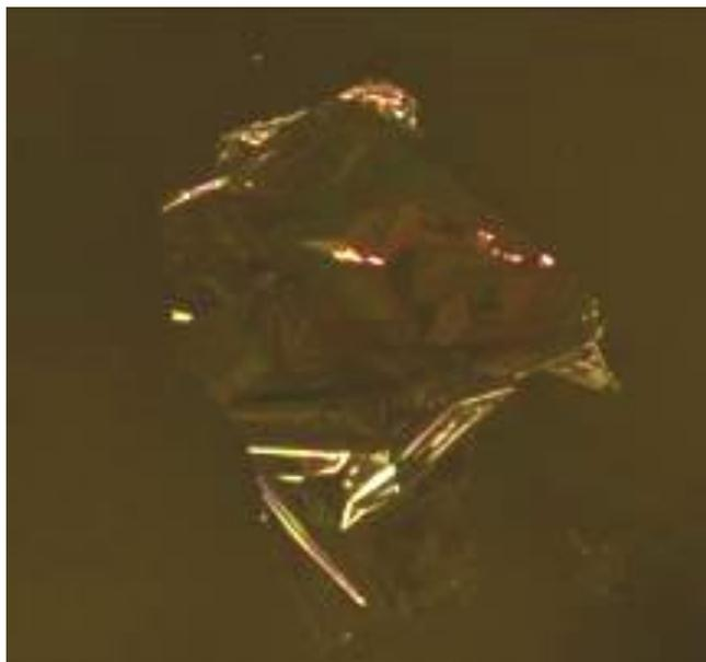
**Figure 5.16** Transparent film formed after evaporating 0.1 g droplet of 5 wt% PAN solution in DMF.
