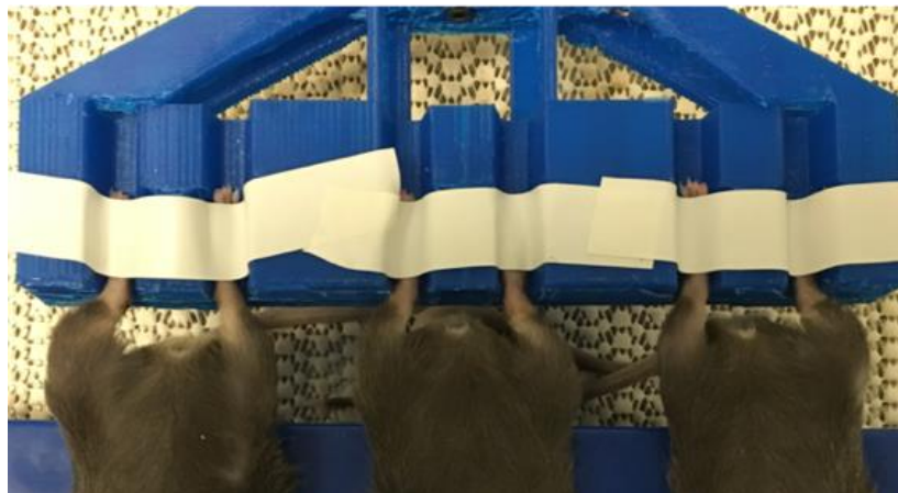
Figure 4.1. Equipment used to deliver local low-intensity vibration (LIV) to mice. Mice were anesthetized and placed in a supine position with their feet attached directly to the actuator of the vibration device. LIV was applied horizontally at 90 Hz with peak acceleration of 0.2 g (amplitude < 0.1 mm) for 30 min/day. The non-vibrated controls were treated identically but were not subjected to LIV.
