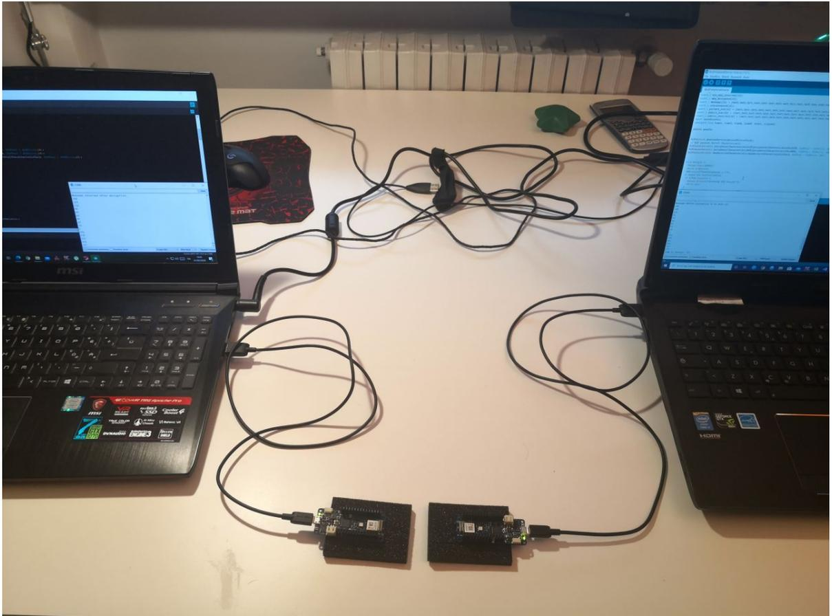
Figure 6: Two Arduino MKR Wifi 1010 boards connected to different PCs and communicating with each other
