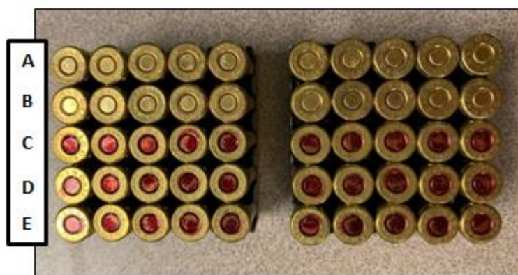
Figure 5: Sellier & Bellot ammunition. Rows A & B were the acetone-cleaned Control Group and rows C, D & E were the Lacquered Group.
